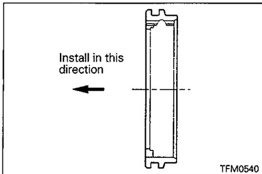
(2) Make sure that the synchronizer sleeve is positioned in correct direction.
