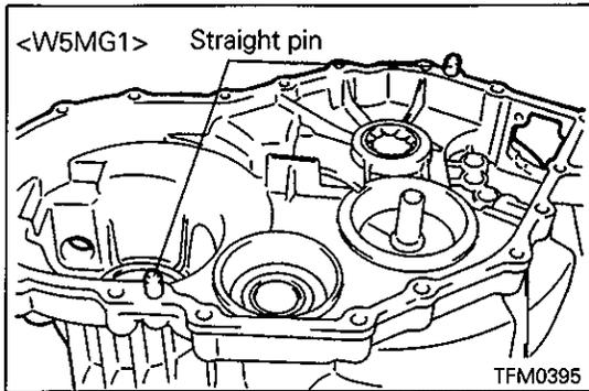
(3) Drive in the straight pins to the positions shown in the illustration. <W5MG1>
