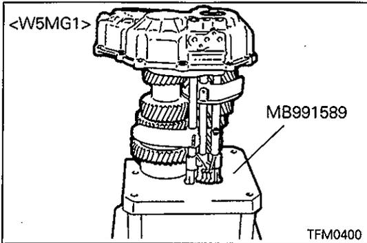
**◆B◆ INPUT SHAFT LOCK BOLT INSTALLATION**
