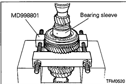
**◁C▷ BEARING SLEEVE REMOVAL**
