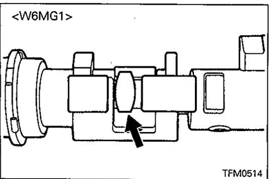
(2) Apply grease to the return spring and attach it to the shift shaft.
