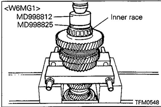
**6. 3RD – 4TH SYNCHRONIZER <W6MG1>****DISASSEMBLY AND REASSEMBLY**
