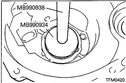
▶M◀ BEARING OUTER RACE INSTALLATION
