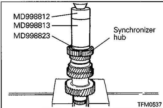
⇨C⇩ **BEARING SLEEVE INSTALLATION**
