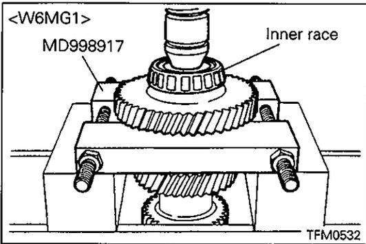
**◁B▷ SYNCHRONIZER SLEEVE REMOVAL**
