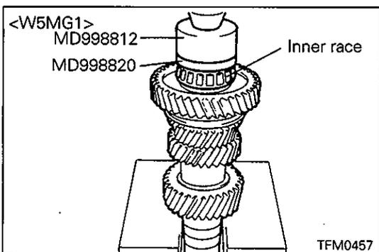
▶◀ BEARING INNER RACE INSTALLATION
