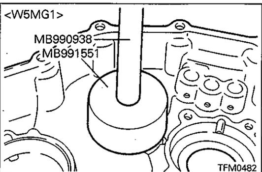
▷C◁ BEARING OUTER RACE INSTALLATION
