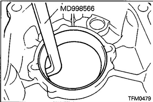
◁B▷ BEARING OUTER RACE REMOVAL
