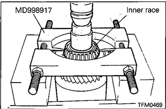
**◊D◊ BEARING INNER RACE REMOVAL**
