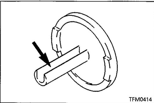
**⇨⇩ INPUT SHAFT REAR SEAL CAP INSTALLATION**
