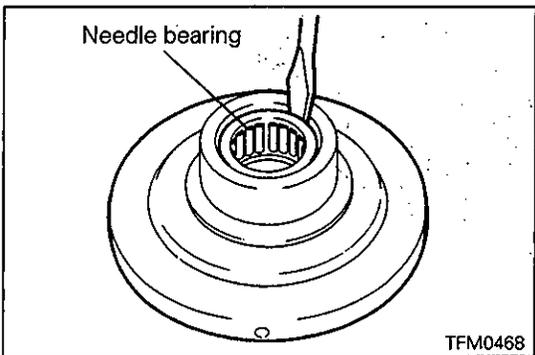
**◊C◊ NEEDLE BEARING REMOVAL**
