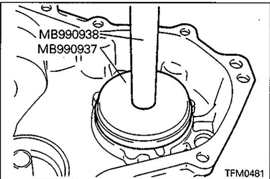
▷B◁ BEARING OUTER RACE INSTALLATION
