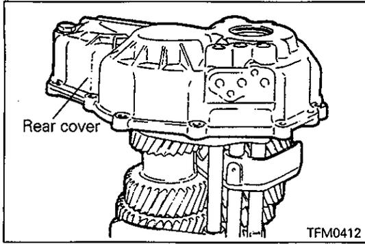
(4) Remove the Special Tool and install the rear cover.
