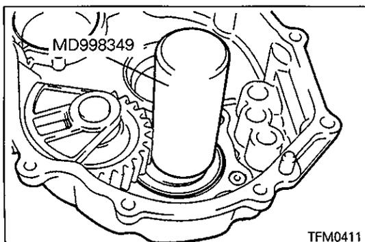
(3) Place the heated Special Tool on the input shaft rear bearing inner race position of the rear cover for approx. 10 minutes.
