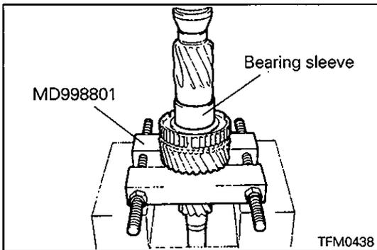
**◁D▷ BEARING SLEEVE REMOVAL**
