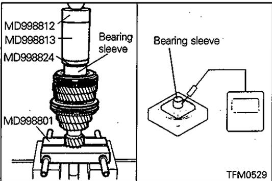
◆K◆ 5TH SPEED GEAR INSTALLATION
