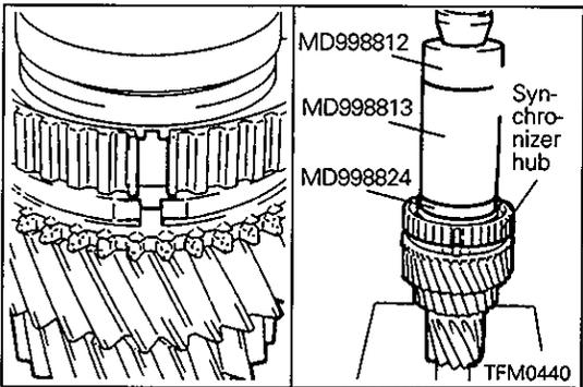
⇄ 3RD – 4TH SPEED SYNCHRONIZER HUB INSTALLATION
