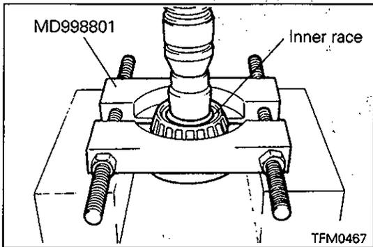
**◊B◊ BEARING INNER RACE REMOVAL**
