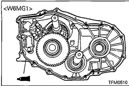
(2) Install the clutch housing.
