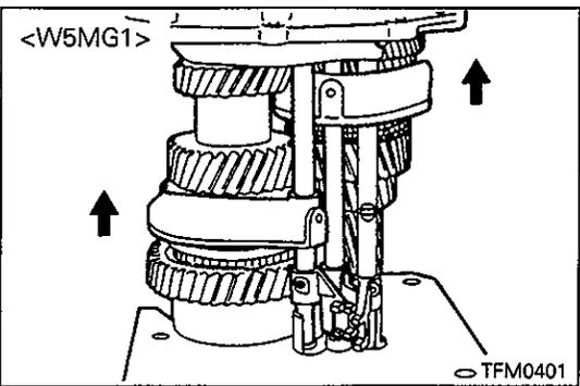
(2) Shift the sleeves as shown in the illustration to engage gears to fix the shaft.
