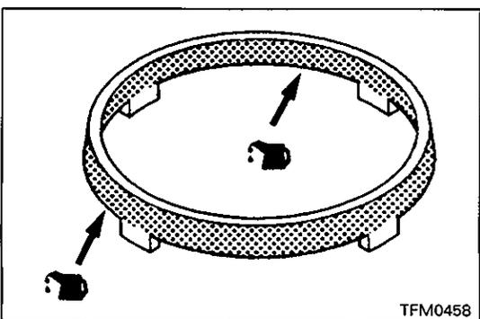
▶◀ SYNCHRONIZER CONE INSTALLATION
