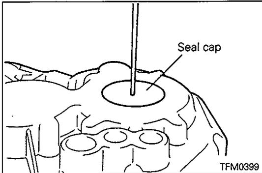
**◁F▷ INPUT SHAFT REAR SEAL CAP REMOVAL**
