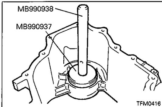
**▶F◀ BEARING OUTER RACE INSTALLATION**
