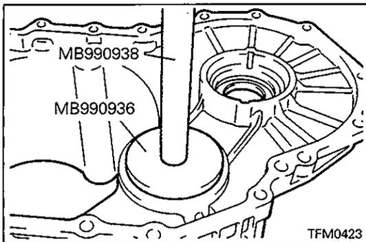
**▶H◀ BEARING OUTER RACE INSTALLATION**
