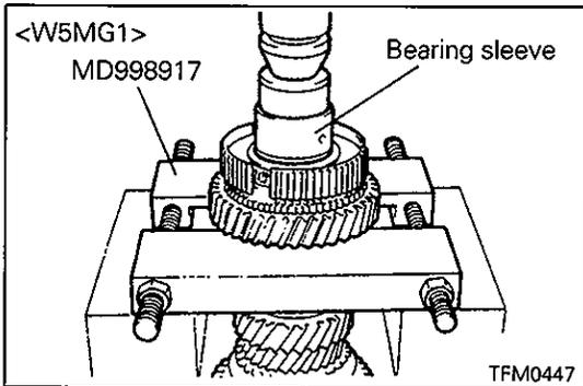
**◁C▷ BEARING SLEEVE REMOVAL**
