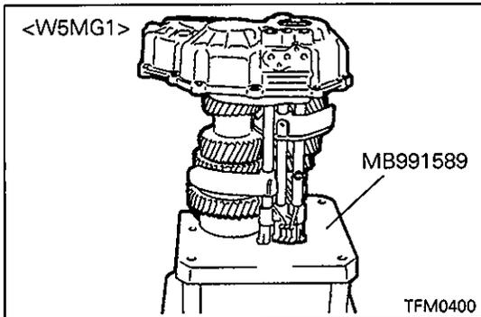
**◁G▷ INPUT SHAFT LOCK BOLT REMOVAL**
