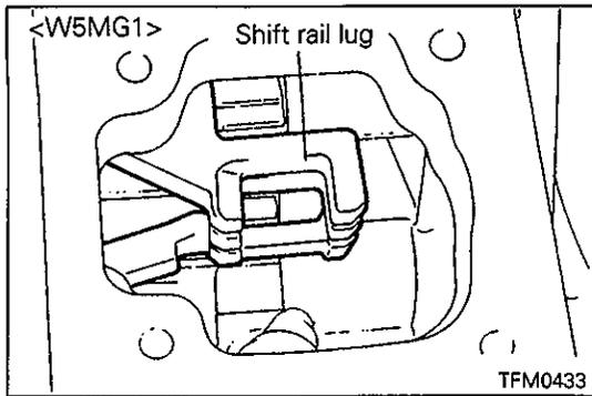
(4) Install the shift shaft while passing its tab in the grooves of shift rail lugs as shown in the illustration.
