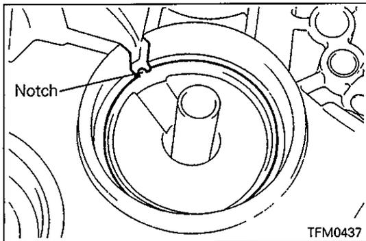
▶O◀ BEARING OUTER RACE INSTALLATION
