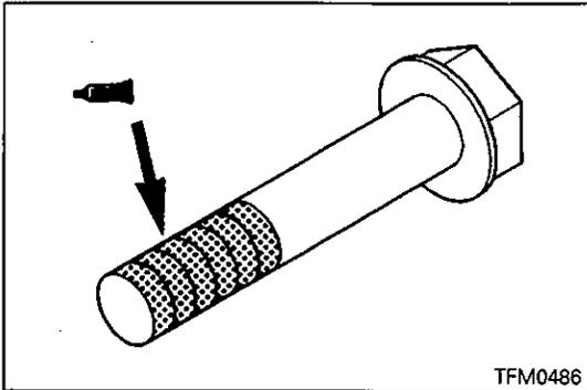
**⇨G⇨ REVERSE IDLER GEAR SHAFT BOLT <W5MG1> / REVERSE IDLER GEAR RETAINER BOLT <W6MG1> INSTALLATION**
