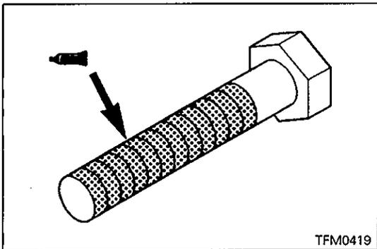
(5) Apply sealant to the bolt threads and tighten the bolts to the specified torque.
