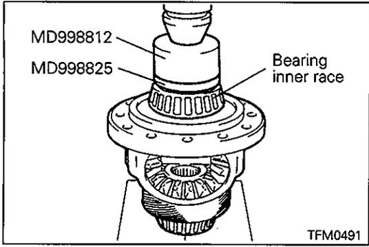
◆B◆ BEARING INNER RACE INSTALLATION
