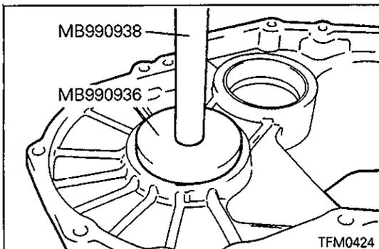
**▶I◀ BEARING OUTER RACE INSTALLATION**
