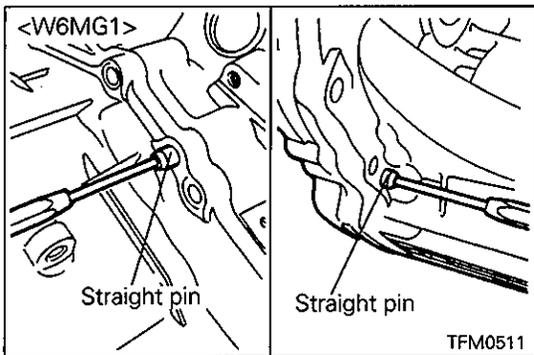
(4) Drive in the straight pin as shown in the illustration. <W6MG1>
