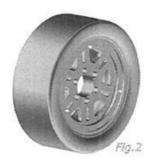
3. Centre the bead of the tire over the stepped bead lock edge. On most applications the tire will fit easily over the step. If the tire bead does not drop over the step easily, apply a liberal amount of soap solution to the bead. Mount the beadlock clamping ring onto the three locating pins. Using a cross hatch pattern, tighten all bolts, in steps of 5nm. at a time, working your way around the clamp until 15nm. is achieved.
