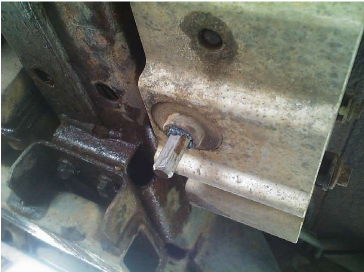
Here below is the hex in the cap an you can see the drive grip has been squeezed out as it was pushed in, so now it should be very snug!!.
