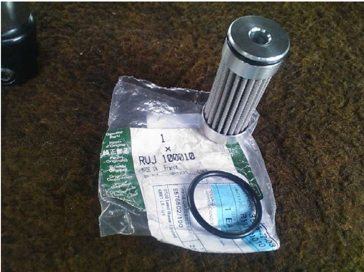
Here's what the new filter looks like, it "should" have an "o"ring on the top of the filter and you will need a new seal for the cap to.
