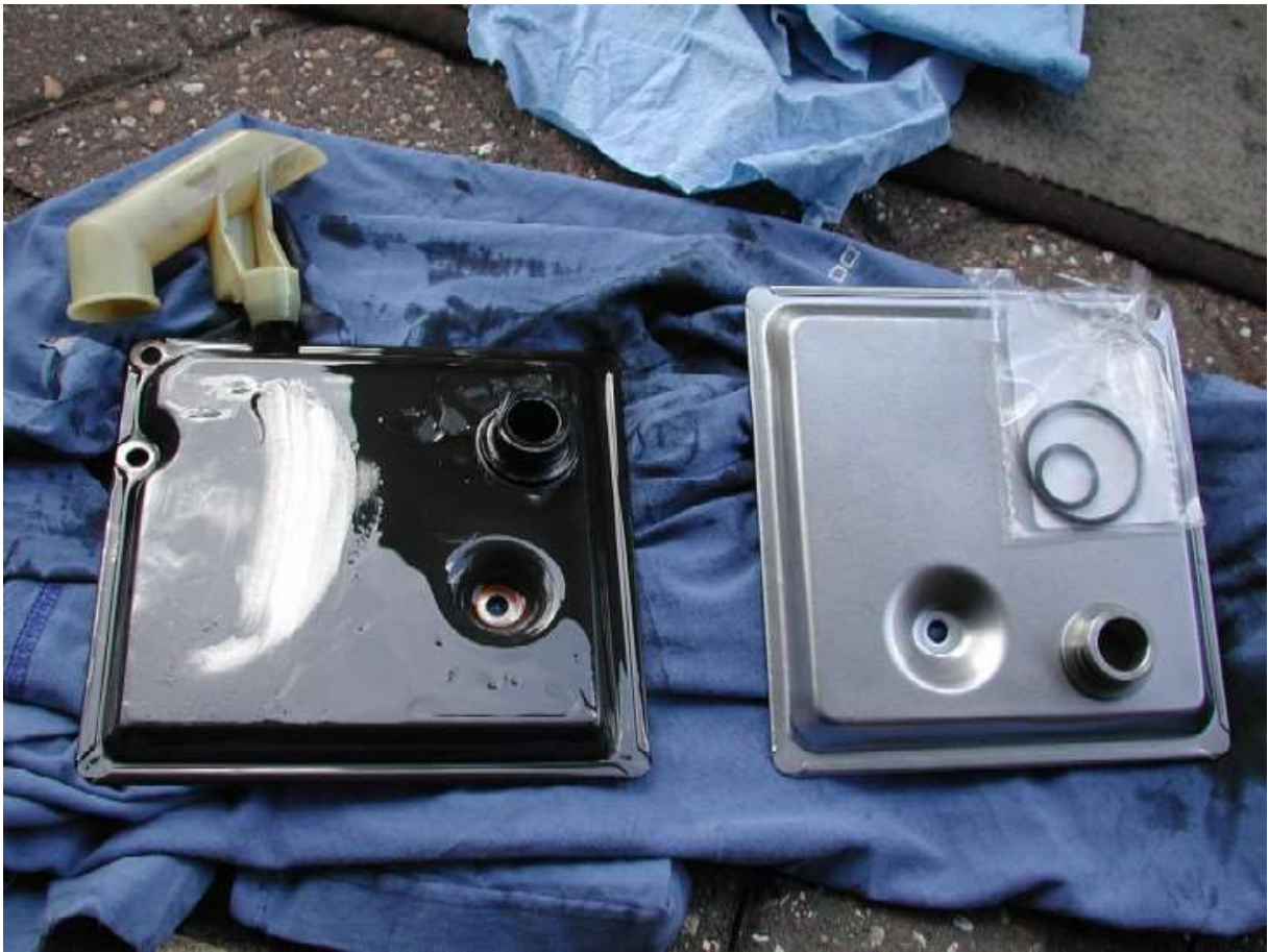
The "pick up" tube simply pops off, there is 2 new "O" rings supplied in the kit. The small one goes under the pick up tube, lubricate the new seals with new ATF fluid.....
