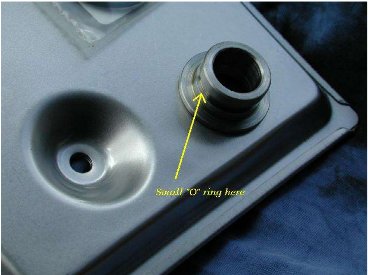
The "pick up" tube simply pops off, there is 2 new "O" rings supplied in the kit. The small one goes under the pick up tube, lubricate the new seals with new ATF fluid.....
