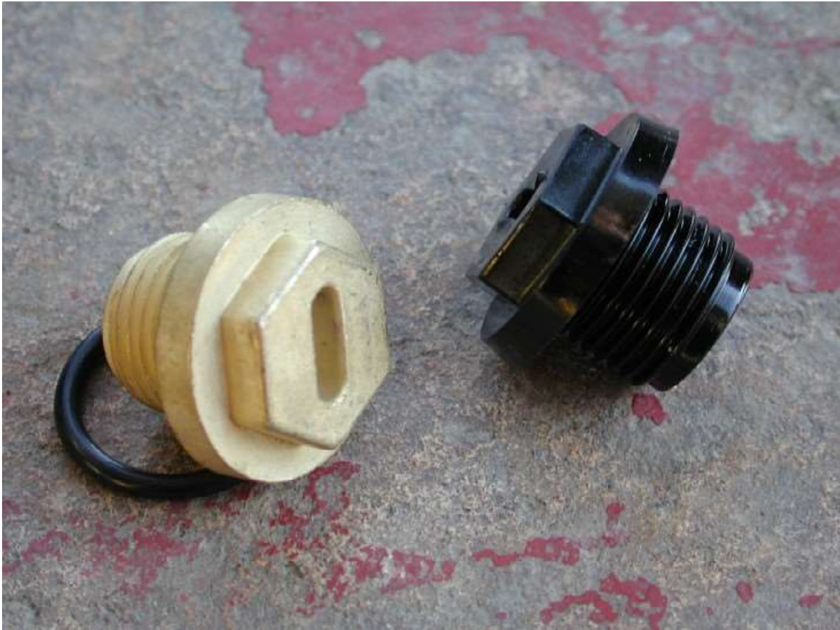
Same plug fits both front and rear diff pans, I simply drove up onto some ramps to change the front one so I did not loose any of the new oil, and reversed up the ramp to change the rear plug to.
