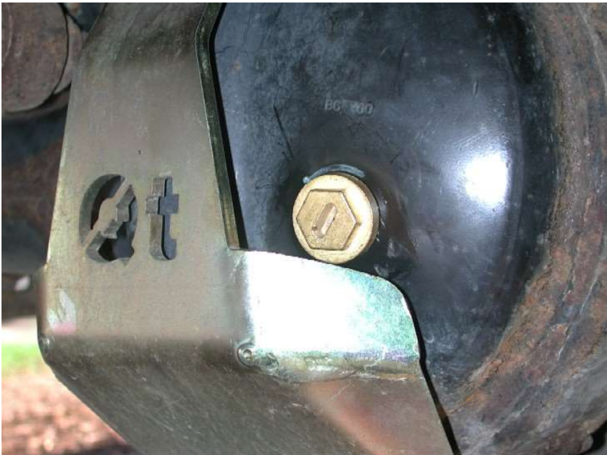
Same plug fits both front and rear diff pans, I simply drove up onto some ramps to change the front one so I did not loose any of the new oil, and reversed up the ramp to change the rear plug to.
