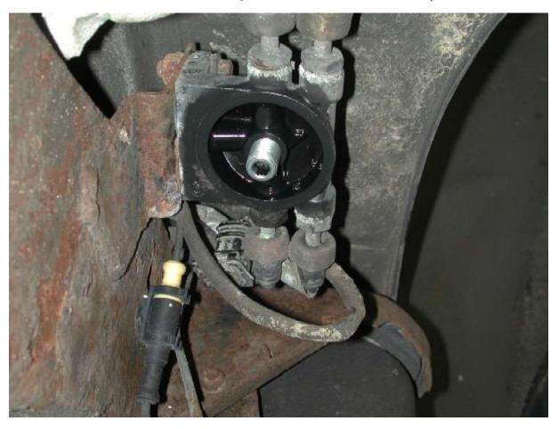
The filter will still be full of fuel even after the initial spillage, so be careful not to turn it upside down or drop it etc.
