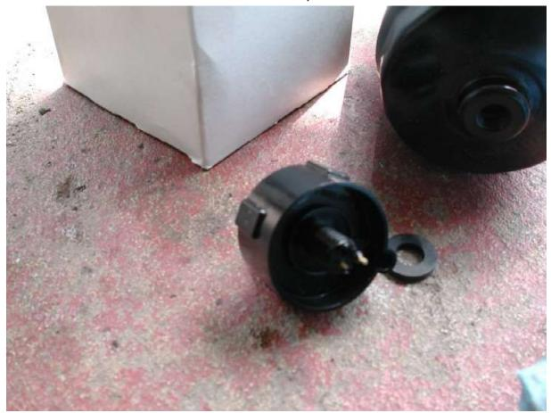
Fit the new seal to the water sensor and screw it into the bottom of the new filter, but only hand tight, do not over tighten it as it will shear off!!
