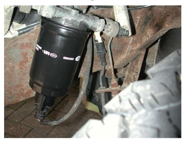
The Fuel Filter also incorporates a water sensor to warn the driver if there is to much water in the fuel by illuminating a light on the dash.
