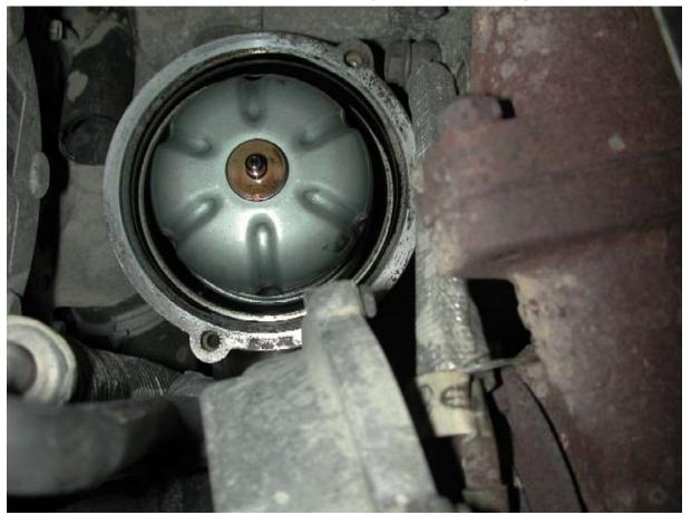
The filter simply "lifts" out of the central spigot, take care to try and not spill any oil on the engine as you remove it. Once the filter is out, use some CLEAN rag or tissue and give the whole housing a clean / wipe out internally as best you can. Make sure you clean the "rim" at the top where the new seal will sit and take care not to drop any dirt or grit in there either.
