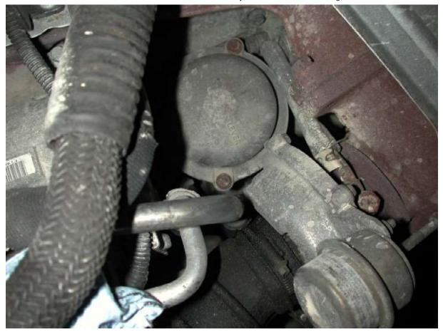
The breather hose / breather valve pipe from the rocker cover runs above the oil filter housing, so to aid clearance simply undo the jubilee clip where it attaches to the turbo hose and move it out of your way.
