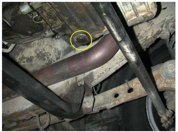
Now depending on how long you left it running, the oil could be warm or VERY hot, so either wear some gloves or be very careful when removing the plug. Its a 17mm spanner size and should not be that tight to remove. I have given up trying to "catch" sump plugs once they almost drop out, so I just let it fall into the bowl and go fishing later on with a magnet, this also help you to avoid getting burnt by the hot oil.
