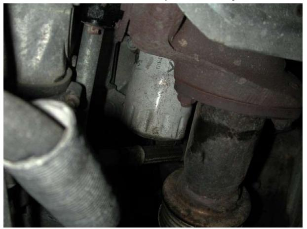
The oil filter should NOT be that tight as they are tightened by hand on installation, use a cloth or rag to help you grip it and undo it slowly. Once its un screwed you will have to tip it and feed it out through the gap you can see above. Some spillage of oil is un avoidable, but you can place a rag or tissue below it first to help soak up as much spillage as possible.
