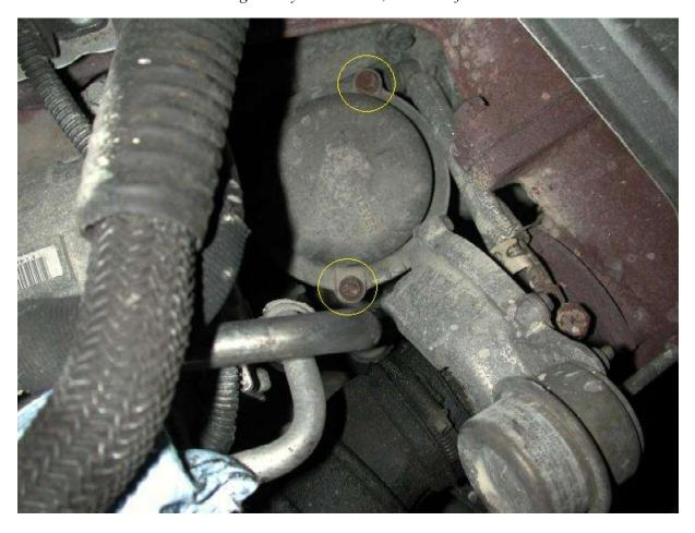
The bolts can stay "captive" to the housing lid, but to make sure they are un done all the way I chose to remove them completely. My lid simply pulled up and off with light pressure. This is what it looks like removed, take note of the black "O" ring seal on the lid.
