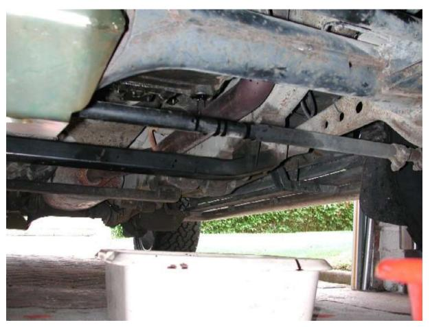
The Sump plug you need to remove is right at the back left corner of the engine sump
