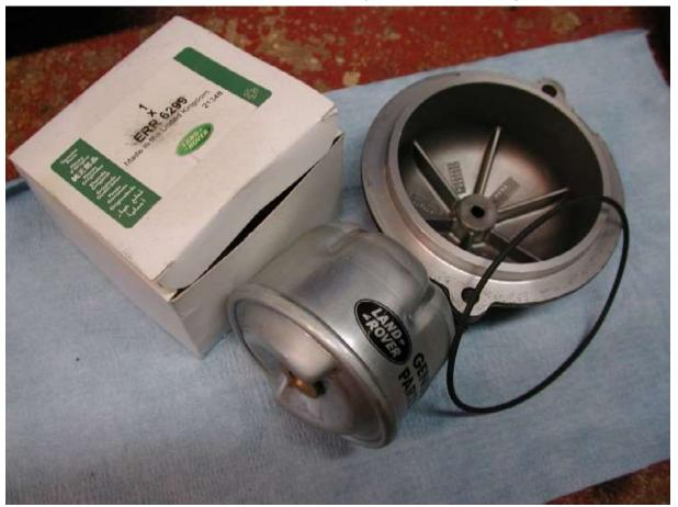
Re-fitting is a reversal of the removal. Smear a "little" fresh new oil onto the seal, fit that to the lid, simply drop in the new filter onto the central spigot, refit the housing lid and tighten the bolts to 10 NM or 7 Lbs FT or 88 Lbs In
