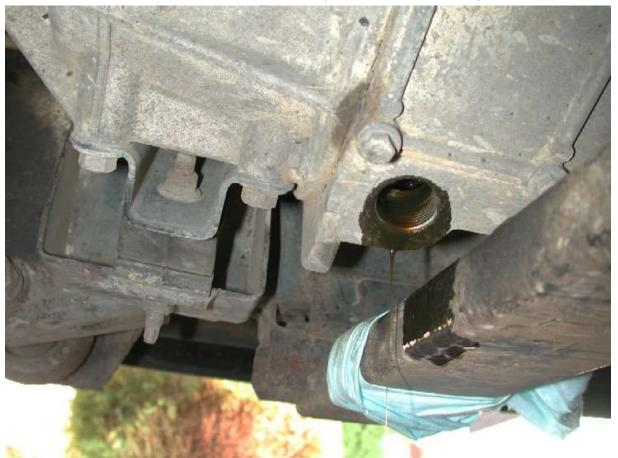
The drain plug is identical to the differential drain plugs in that it contains a magnet to collect any metal particles in the transfer box. You will see "some" stuff on there but not to much (I hope).
