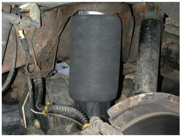
If all is good, restart the car and allow the compressor to run its full cycle to inflate the bags up to working pressure. Once it has stopped, refit the road wheels, you may have to adjust the axle height by using the 2 jacks to allow the wheels to be refitted.
