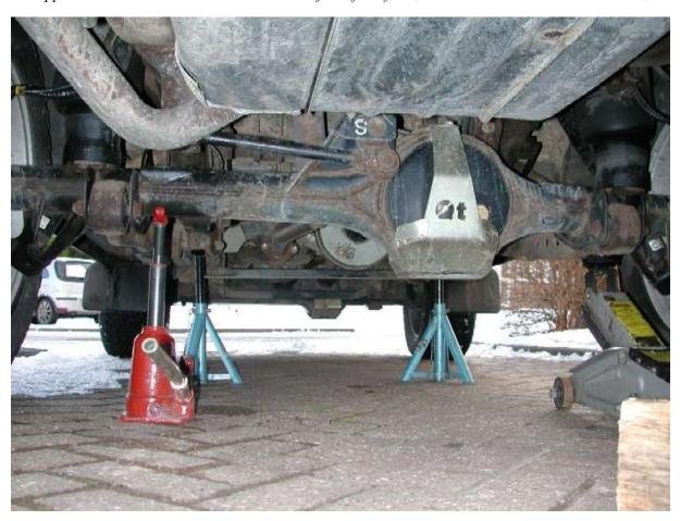
Next we have to somehow de-pressurize the Air springs, below you can see there is a 10mm connection union on top of each air spring, but because of where it is, its difficult to get a spanner in there to undo them, so its easier to let the air pressure out at the compressor end.
