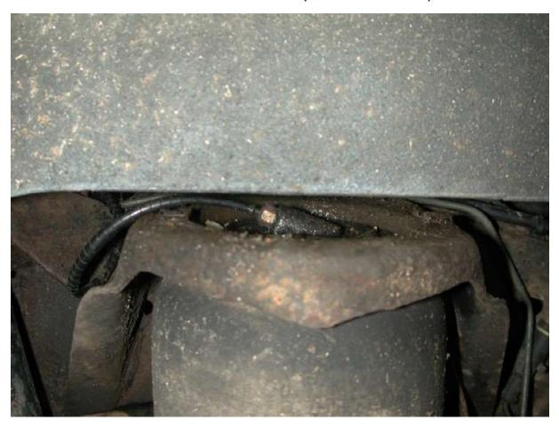
Under the vehicle level with the front passenger seat (UK car) the suspension compressor assy is housed in a small plastic box bolted to the outside of the left hand chassis rail. It has 2 "Zeus" quick release fasteners that once undone allow you to lift of the cover. Once the cover is off, a the front of the compressor assy you will see 3 unions / air pipes. We are ONLY interested in the outside 2 pipes NOT the middle one
