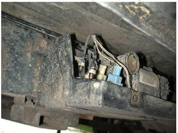
They are also 10mm in size, one at a time, undo them slowly and allow the air pressure to escape, once the "hissing" stops, you can simply check by squeezing each air spring, if its fully depressurized it will squash easily. Take care not to get any dirt on the pipe unions and into the compressor assy itself
