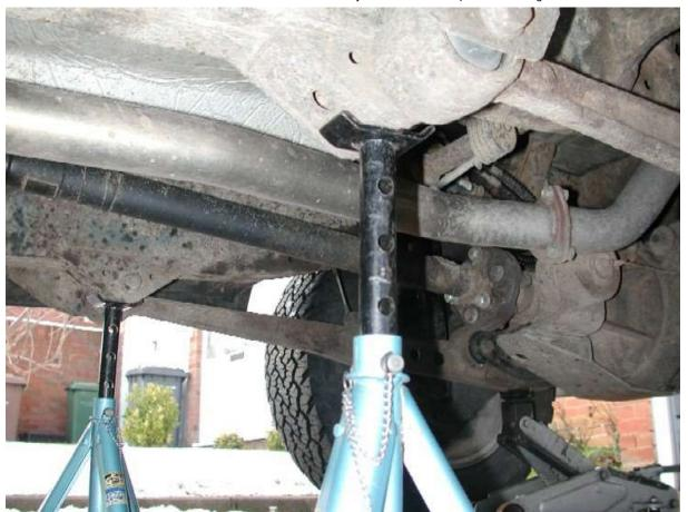
Then get 2 jacks, either trolley or bottle, I used my trolley jack and the vehicle bottle jack, lift and support the rear axle so the rear wheels are just of the floor, and then remove both rear wheels,
