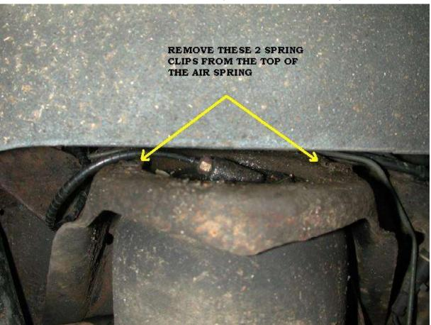
I found its easiest to just remove them carefully with a flat bladed screwdriver, try not to loose them if you don't have new ones ready!! Picture below for ref the spring clips (air spring out)
