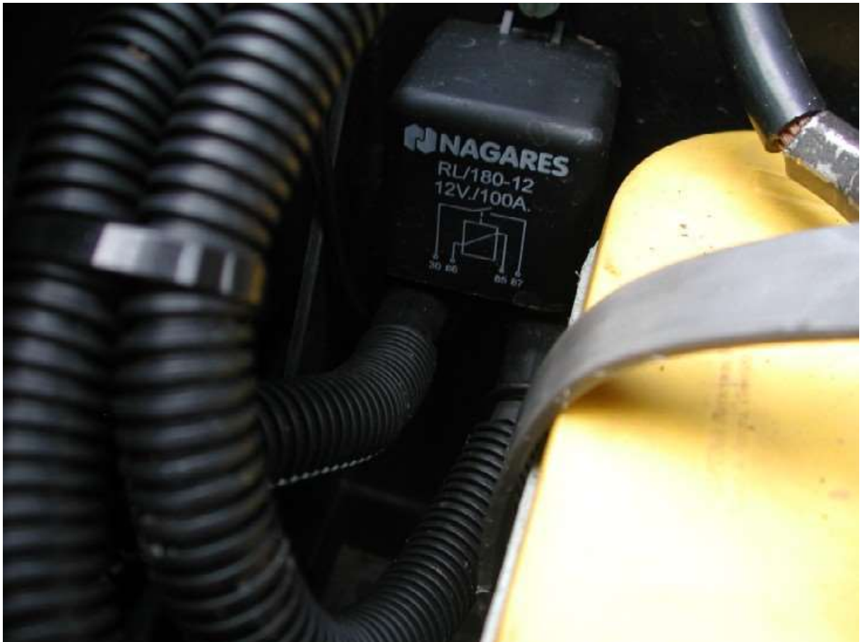
With the tray now fully installed, the split charge relay was mounted where the single Albright was.....
