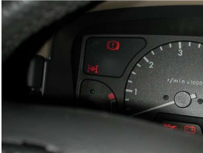
Diff lock Light on the Instrument Cluster
