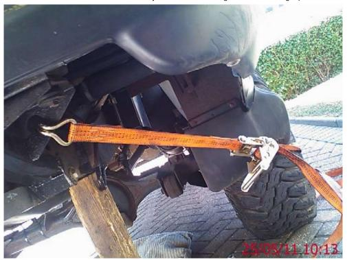
Once these outer bolts are slaved in, then slave in the central pivot bolt and nut (the big one)
