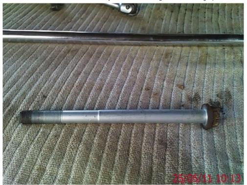
After the central bolt is out, you can then pivot / wiggle the watts linkage to remove the assy from the car...
