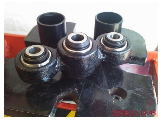
The refit is a reverse of the removal. I used anti seize grease on ALL bolts before re-assembling the link back together.
