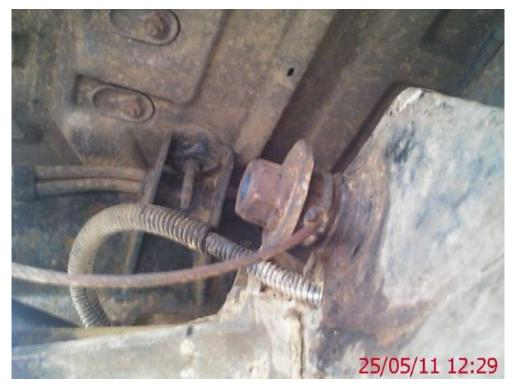
So remove the 24mm nut, then the washer and lanyard and you can then access the central pivot bolt nut. This bolt is torque'd to 170lbs ft, so its quite tight to undo. Once that's undone, remove what is probably the longest bolt on the car!!!
