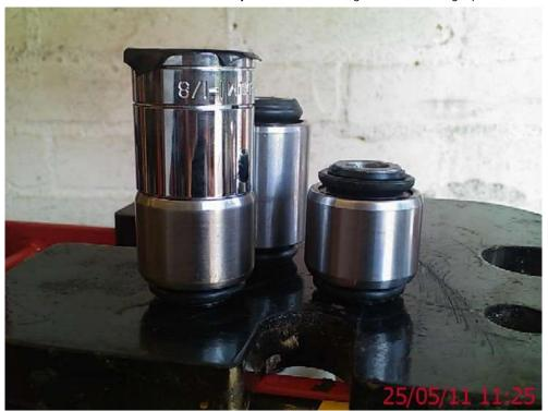
Push the new central bearing and outer bushes into the pivot link so they protrude equally out each side.
