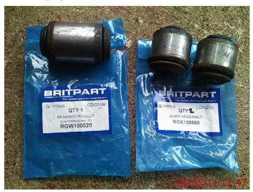
Now you can use the same socket for fitting as removal, just "feed" the socket over / around the rubber on the new bush carefully first...
