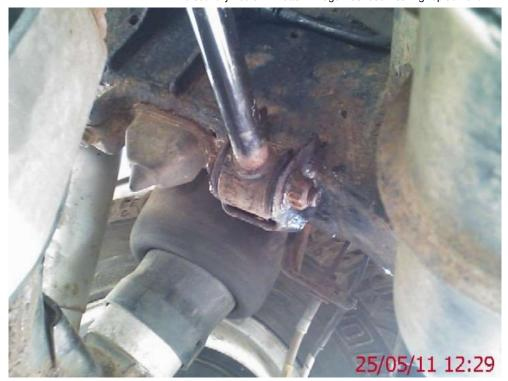
NOTE: - These are what keeps the axle and the body central to each other, once you remove the bolts from these if the vehicle is not on level ground it can move sideways!!
