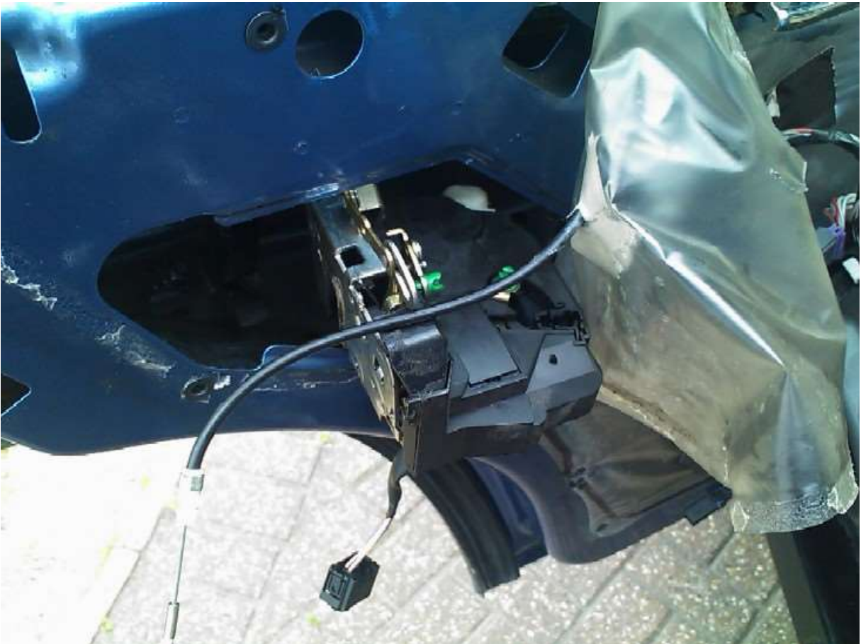
This now gives you enough room to squeeze the lock assy past the frame and out of the hole in the door...(picture shows interior handle cable disconnected)
