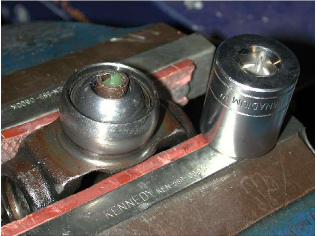
I again used the socket to fit the dust seal "carefully" and then packed it full with new grease.
