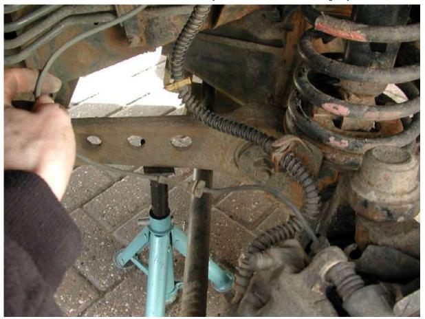
Then lift the caliper away and rest it on the radius arm, take care not to kink or damage the brake pipe. You may need to remove the brake pads and store them safely out the way.
