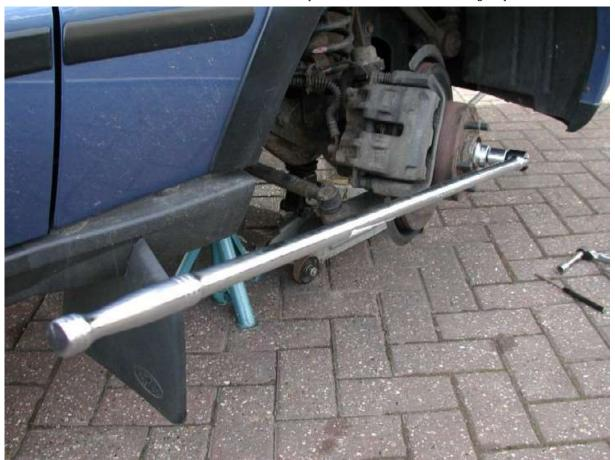
You just need to "break" the torque for now and undo 1 or 2 turns. Now you need to remove the brake calipers and brake disc as well. For "full" info on that check <u>front disc / pad</u> replacement article. For a quick guide, you need to first remove the pad carrying part of the caliper, undo the 2 bolts at the caliper sliders.
