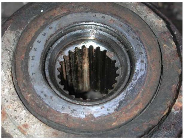
The movement in the bearing was very minimal when off the car, but obviously when you hang a large wheel off it, the movement is "magnified" and it feels a lot worse.
