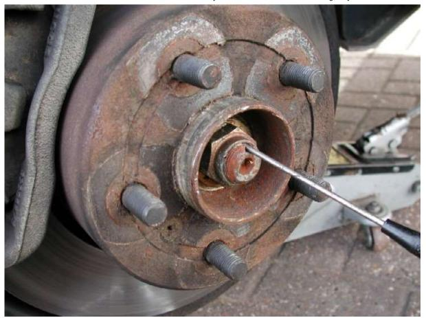
Here lies the first issue, you need to "break" the torque on the nut. I m pretty sure its supposed to be 32mm, how ever I found that size just a little to "sloppy" for my liking with such a high torque, so I used an 1-1/4" AF 6 point socket as it just fitted better. Its about 0.025" smaller than 32mm and that seems to make all the difference. I would HIGHLY recommend you use a 6 point socket as to avoid the possibility of "rounding" the nut off.
