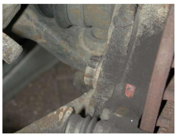
Now you can remove the brake disc by undoing the brake securing screw and then lifting of the disc. If your discs have been of recently then they should come off pretty easily, if not, then spray some penetrating oil around he centre part of the disc / hub and let it soak for a bit. Then if need use a block of wood and give the disc a little help with a hammer to remove it.
