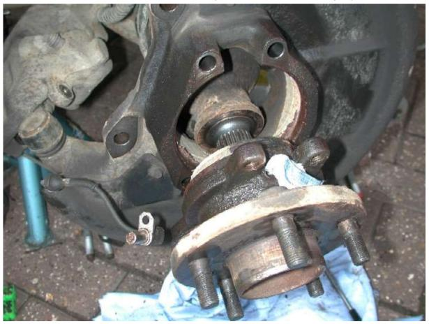
Feed the hub of the drive shaft and also feed out the ABS wiring loom.
