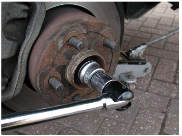
As well as a big torque wrench for refit, you really need a good breaker bar to undo it in the first place. I used a 3/4 drive 1.2m bar and even then it had some force applied before the nut come undone. Turn the wheel so it brings you away from the car when undoing the nut.
