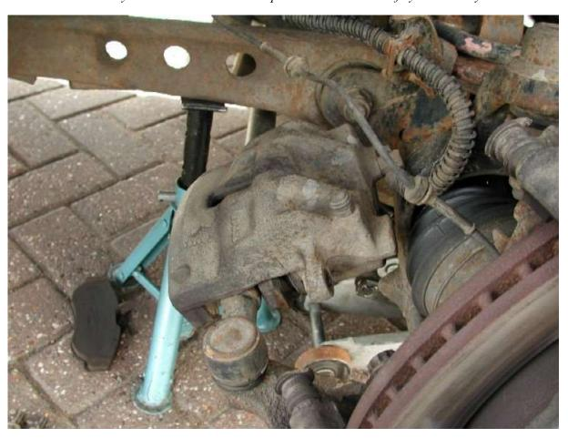
Next you have to remove the inner part of the caliper, that's held on by the 2 12 point bolts that you can now see at the back of the hub.
