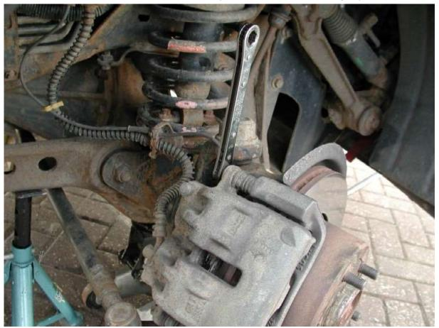
Then before you lift the caliper away, unclip the ABS sensor loom from all the points up to the inner wheel arch. Then go into the engine bay and follow the loom to the connector on the inner wheel arch. It is just below the brake master cylinder on my TD5 (UK car). Feed the loom back out under the wheel arch and leave it there for now.
