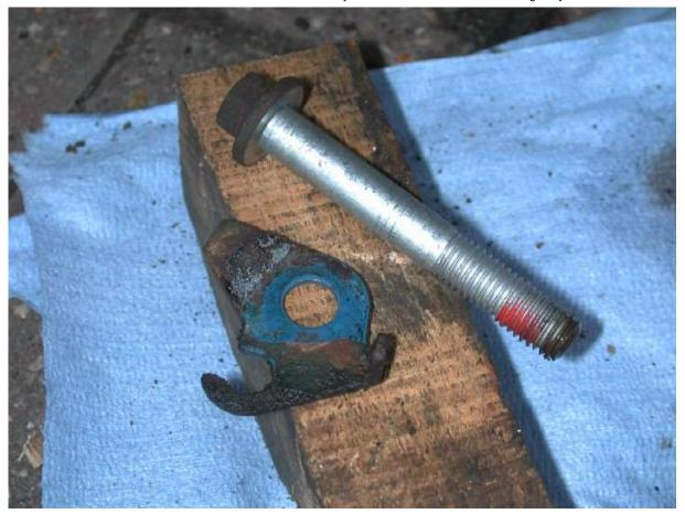
Now you cab remove the Hub Stake nut completely.
