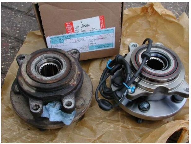
As you can see the new Hub assy comes complete with a new ABS sensor and wiring loom already installed. DO NOT disturb / remove the sensor!!!
