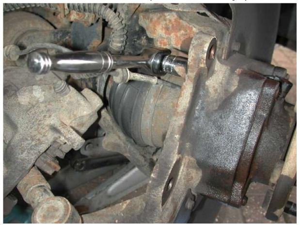
You will need to turn the wheel each way to get access to either the front or rear bolts, be careful of the brake caliper resting on the steering arm when doing this. As with the Hub nut, 6 pointed sockets are always advisable on items like brakes as they get treated to all the elements and are usually rather tight / corroded to come undone.
