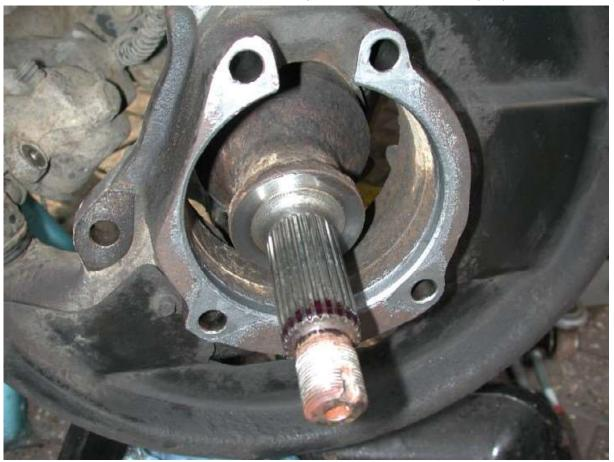
When your ready to start the re-assembly, you need to apply a 3mm wide bead of loctite 640 (or threadlock) as above to the very end of the driveshaft. This will then be smeared down to the splines as you push the new hub assy on. Make sure your have all your tools and bits ready at hand as the Hub assy must be refitted and finally torqued up BEFORE the Loctite goes off!!
