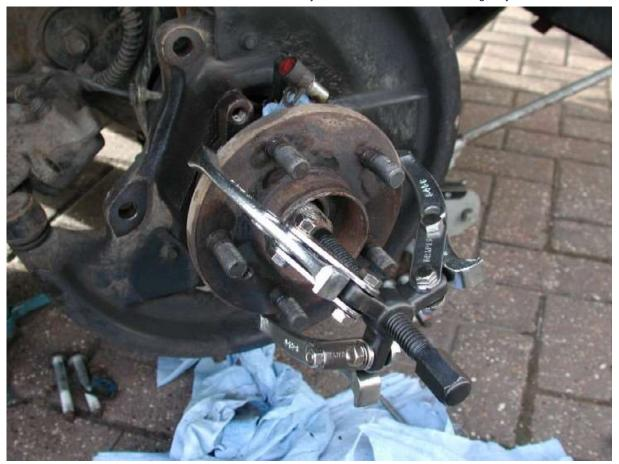
So with a combination of the hammer on the rear of the hub, and the puller, the hub assy came away nicely both from the steering knuckle and the drive shaft and there is no need to replace / disturb any oil seals etc; o)
