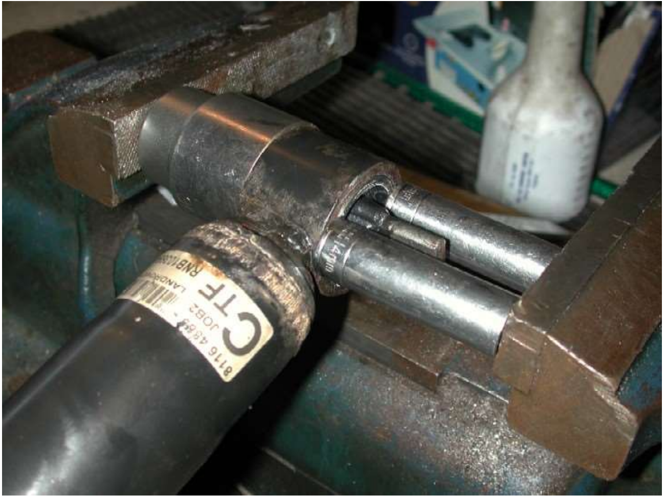
New bush fitted and flush with the shock.
