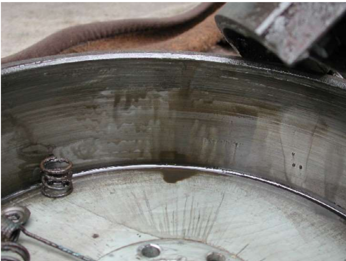
Now I cleaned up all the brake parts using some solvent cleaner ready for refit after the output seal is replaced.
