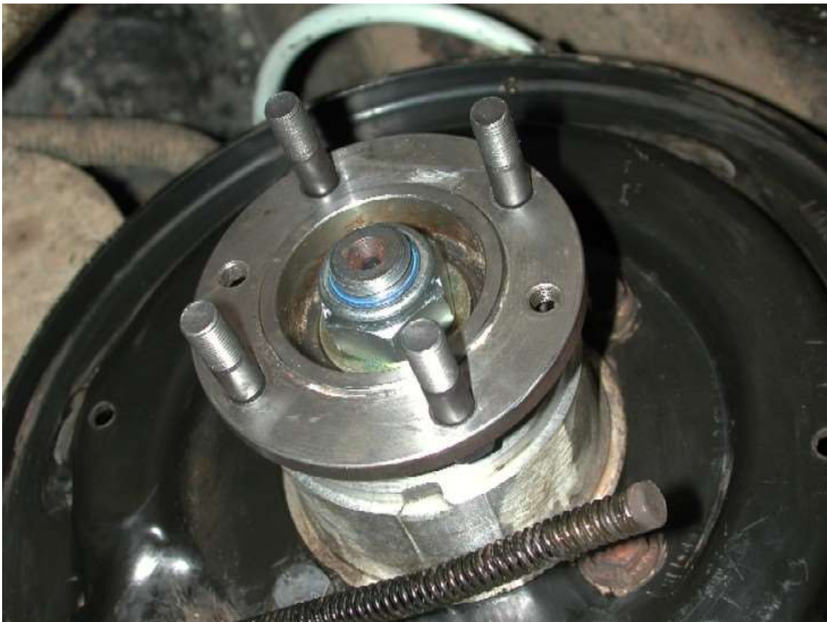
The rest of the refit is a reverse of the removal, if your only doing the seal then its relatively simple, if you need to replace the handbrake shoes, then take care when fitting all the springs etc back in, its fiddly and puts up a fight, but take your time, a second pair of hands may be of some help!!!
