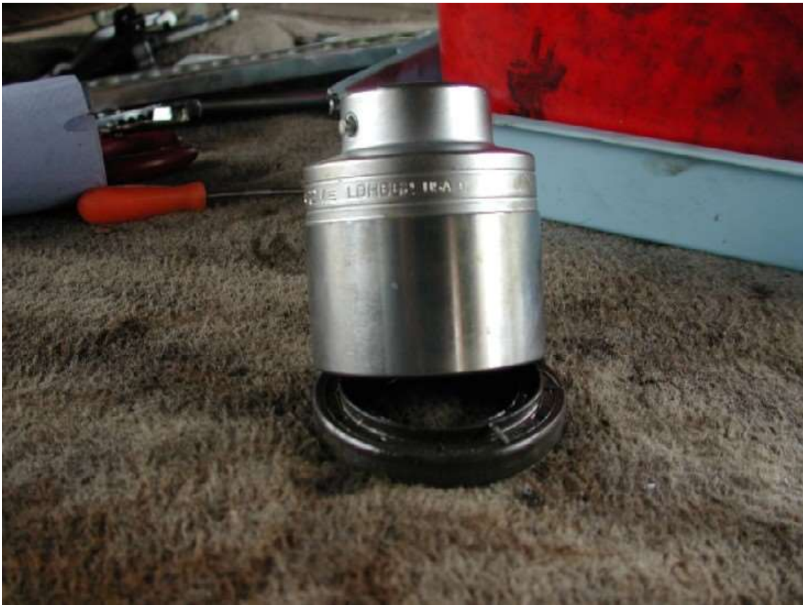
New seal driven into place CAREFULLY as not a lot of force is needed!!!!
