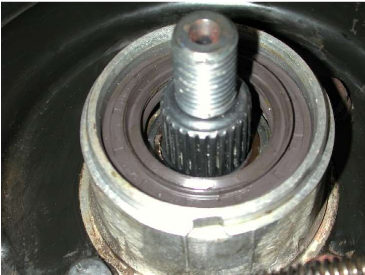
Now refit the output flange and ensure it goes fully home!! then pop in a new fibre washer and make sure that is fully pushed in so its flush with the inner surface.
