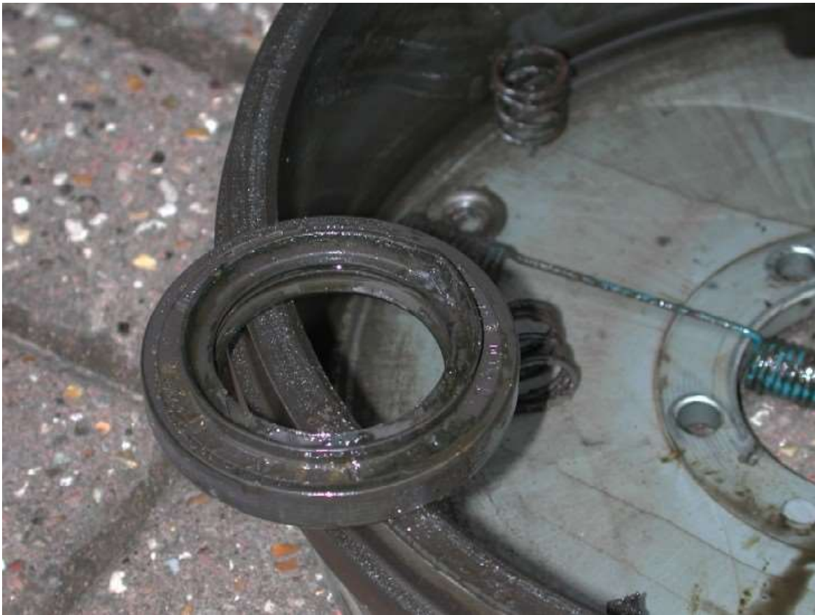
Here below is the seal removed and the handbrake cable is also visible (shoe replacement only), the back plate is all cleaned up of old oil and muck and care was taken to not get any dirt etc into the transfer box
