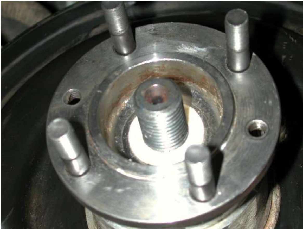
Refit a new spacer / washer and NEW locknut and tighten to 109 Lbs ft
