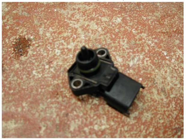
Once its all clean and dry re-fit the sensor to the intake manifold and then connect its electrical plug back up.
