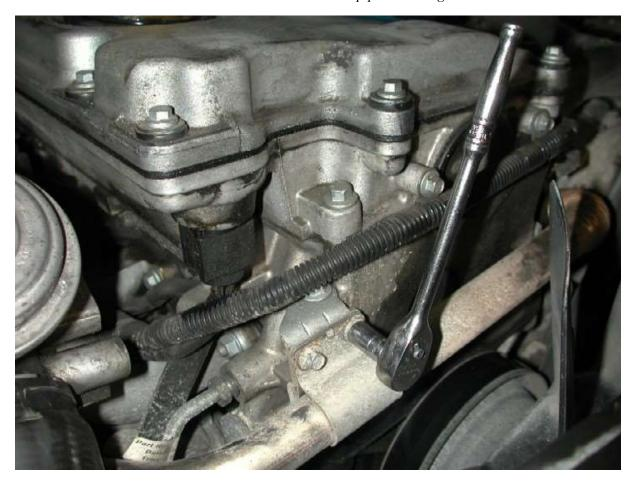
Now remove the 4 bolts that secure the EGR valve to the intake manifold. These should not be that tight and are pretty easy to get on to. After they are out, you now have to remove the 2 allen head bolts that secure the pipe to the exhaust manifold. These have been know to shear of, so its a good idea to soak them in some penetrating fluid or WD 40 etc before you tackle them.
