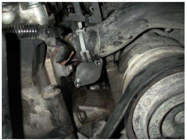
Next is the replacement pipe to go where the EGR valve was. Again I used some new stainless bolts / spring washers, but the original bolts can be re-used here with no problems at all. I did fit a new gasket here, and advise you fit all 4 bolts loosely again before tightening them up.
