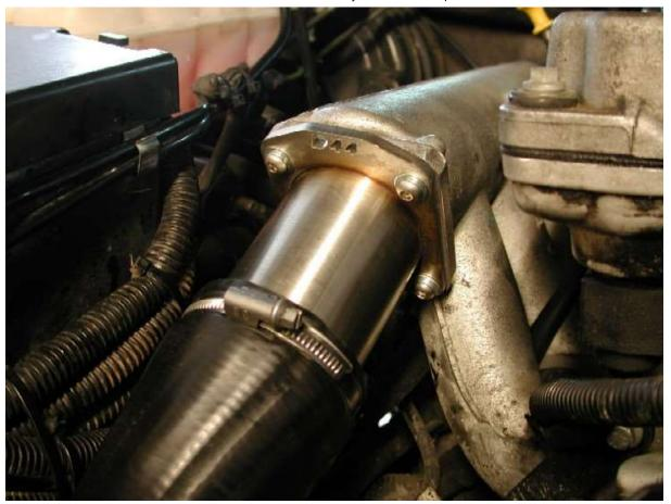
Once the pipe is in, refit the intercooler hose and jubilee clip.
