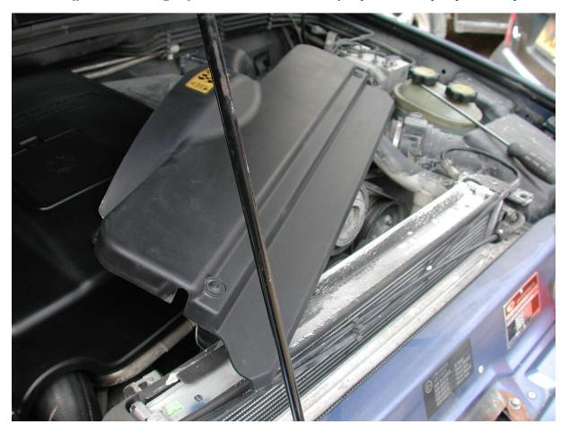
Then the engine acoustic cover, Its held on by 3 bolts, 2 on the passenger side and 1 on the driver side
