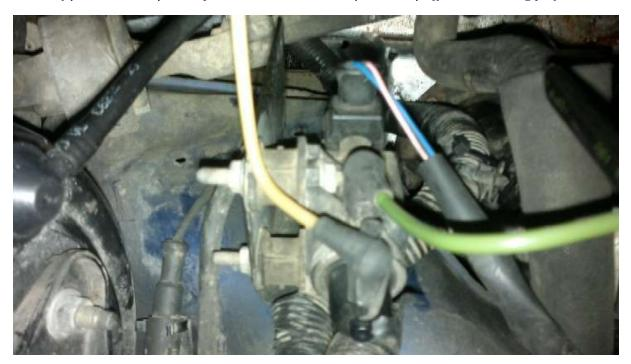
ABOVE you can see the blank installed where the BLUE pipe to the EGR valve was.
