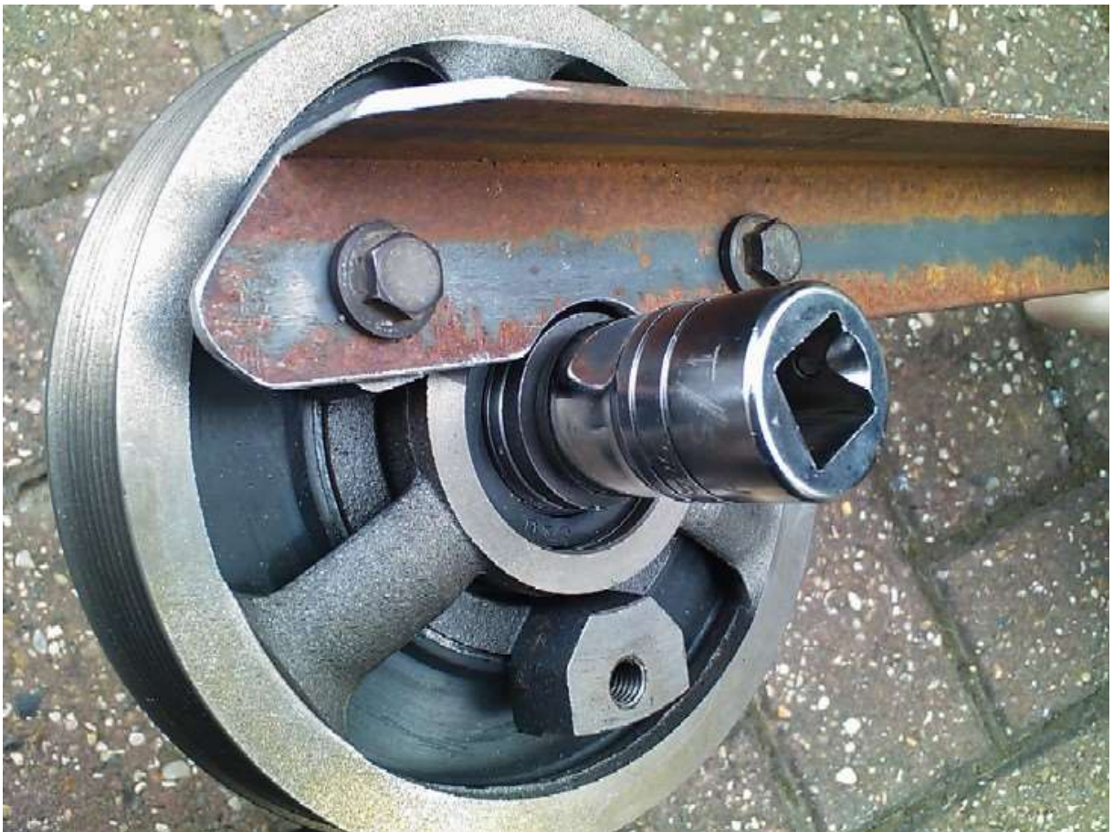
Using the old damper bolts.....you can see the "cutout" to allow the socket and washer on the bolt to pass.
