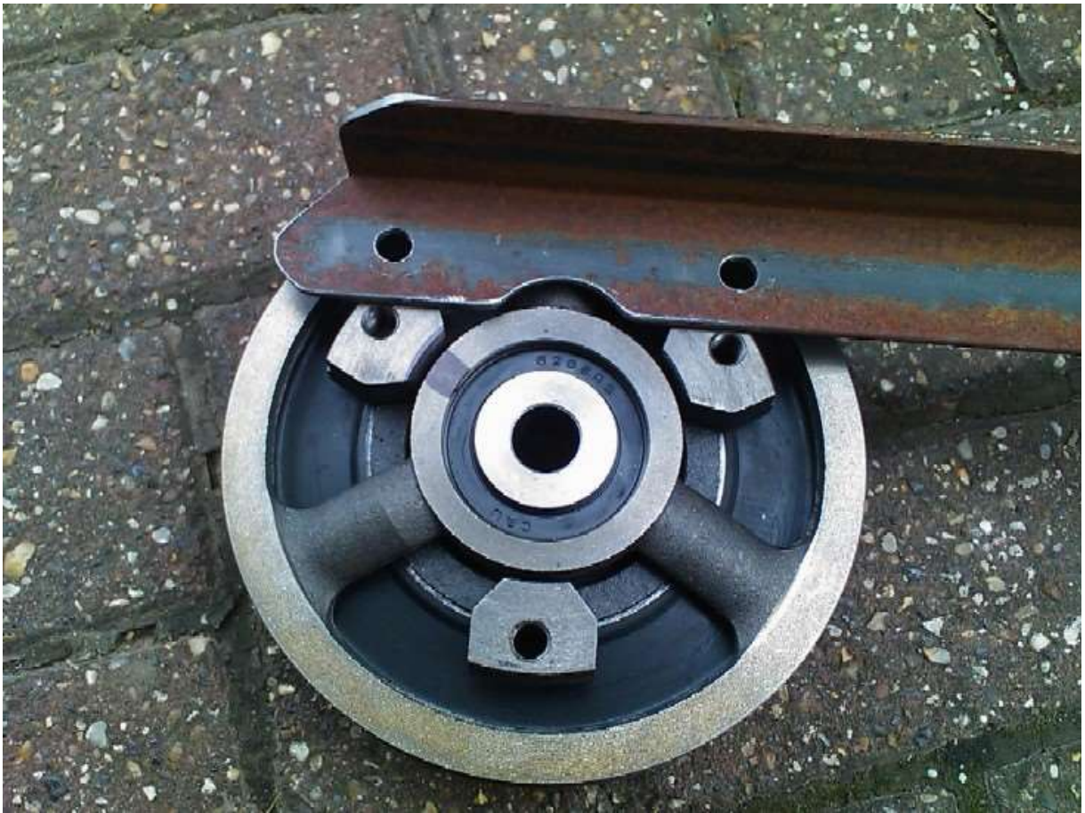
Using the old damper bolts.....you can see the "cutout" to allow the socket and washer on the bolt to pass.
