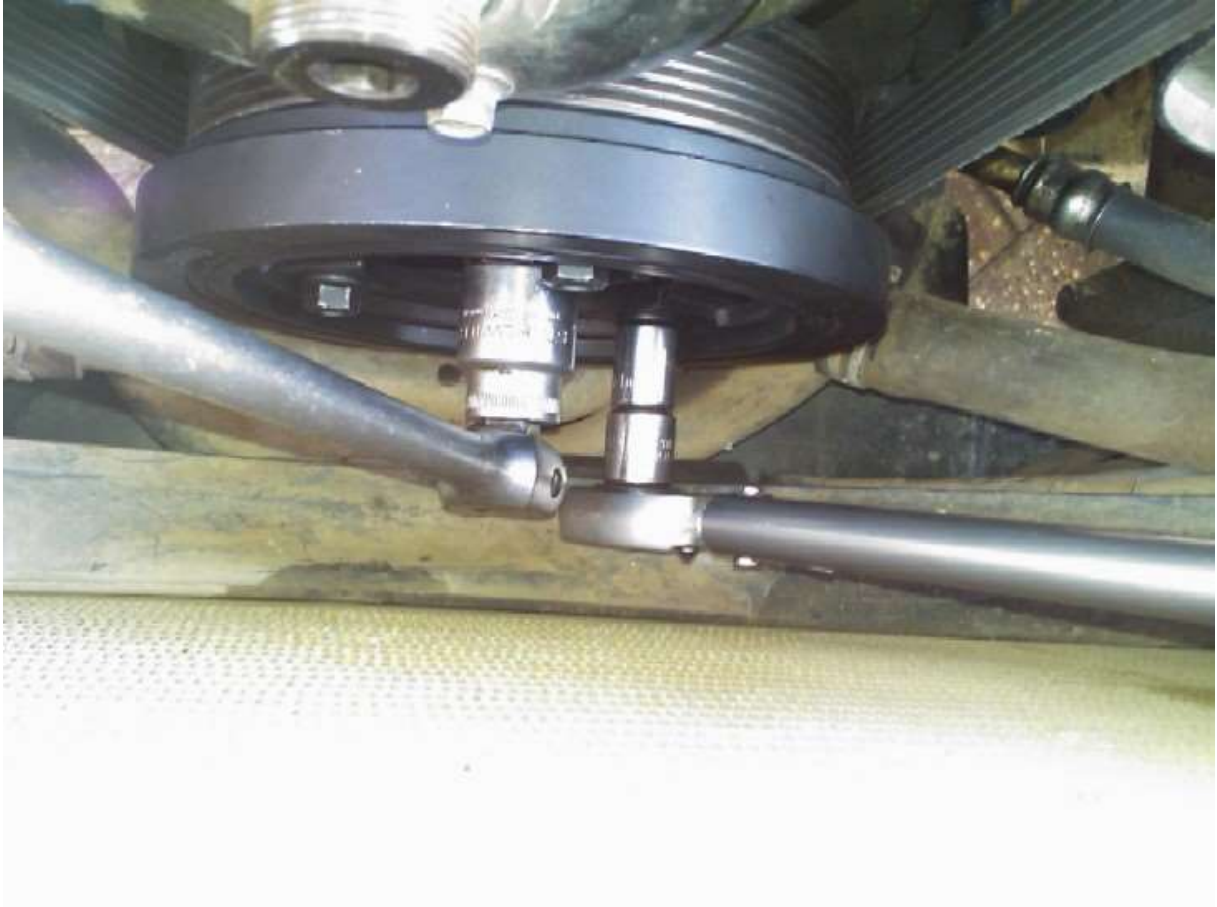
New damper installed, and no more "marble rattle" ;o)
