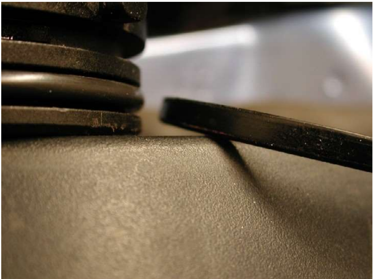
Here below you can see the new "o" ring in place on the end cap, and the old "flat" one next to it !!
