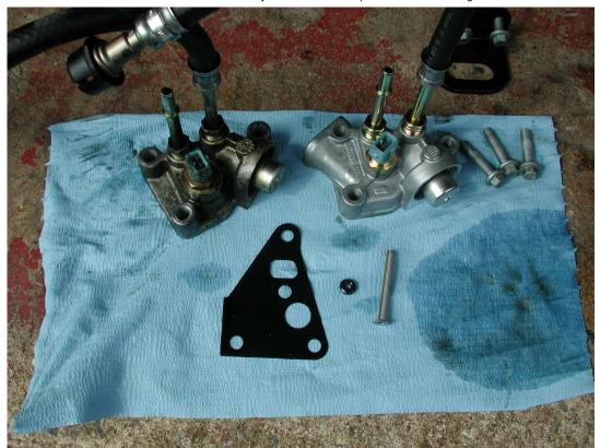
Here you can see the 2 FPR's next to each other, The bolt pattern obviously is the same, but the new modified one has an additional part of the cast where the extra pipe for the external fuel return goes on the later models with 15P engines. You can also see the gasket, "o" ring and the tiny gauze fuel filter.
