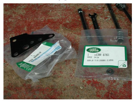
The new gasket is a "crushable" type, and because of the bolt pattern, if its lined up with the bolt holes, then it can only be correct way round
