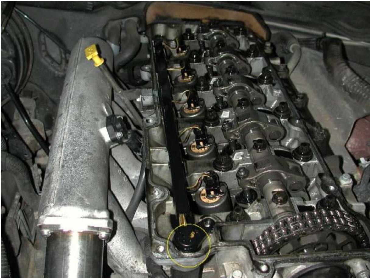
You simply now have to disconnect each plug off the 5 injectors,
