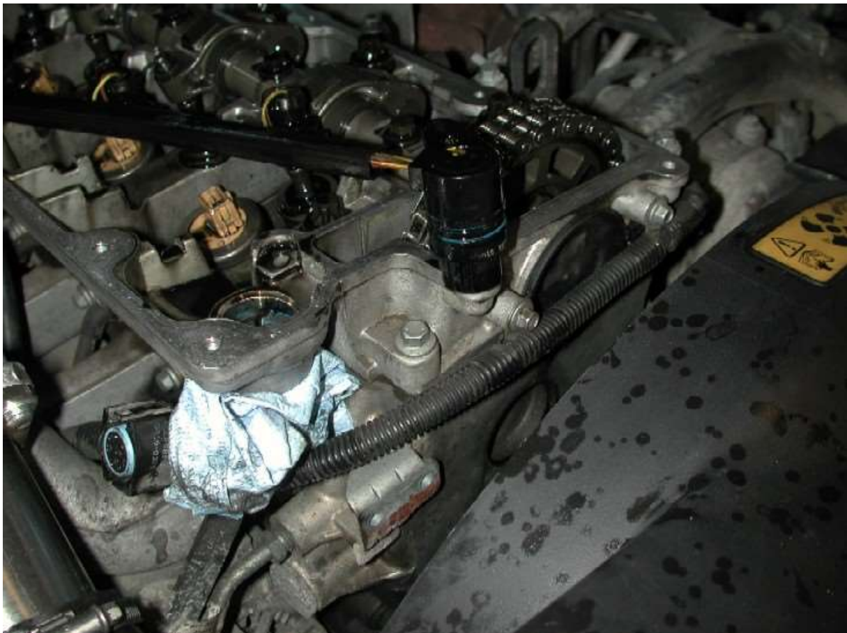
You simply now have to disconnect each plug off the 5 injectors,
