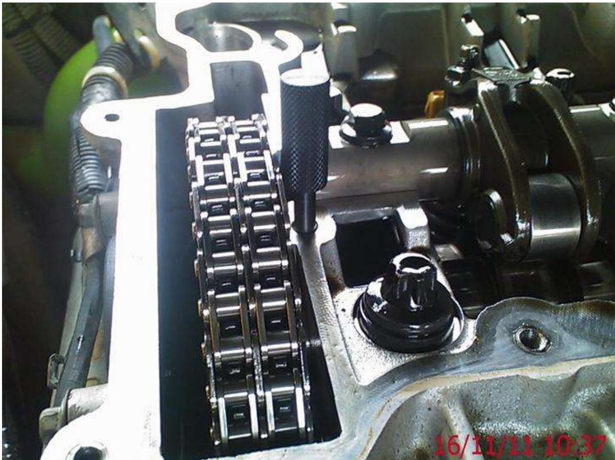
The slot in the pulley is there to line up with the hole above it drilled into the rocker box, this is where you fit a "timing pin" through the hole to lock the camshaft in this position....
