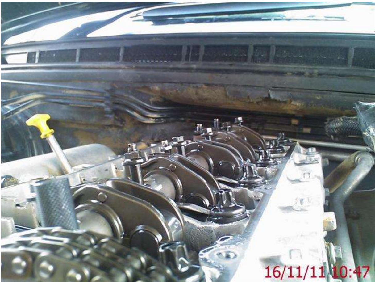
Again the bolts retaining the rocker shaft should be discarded and replaced.....you decide.....
