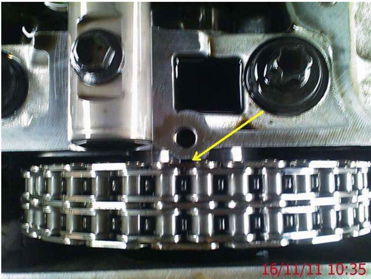
The slot in the pulley is there to line up with the hole above it drilled into the rocker box, this is where you fit a "timing pin" through the hole to lock the camshaft in this position....
