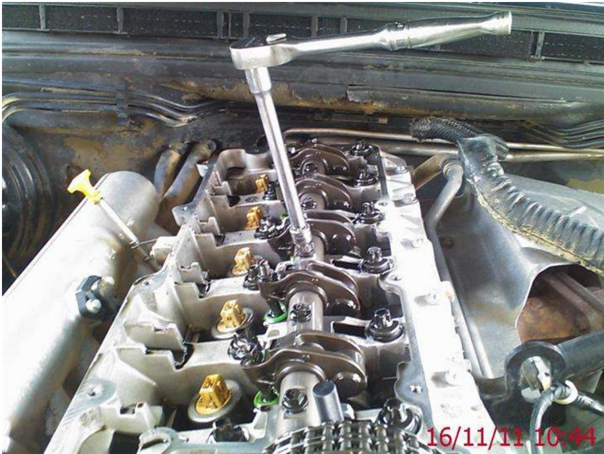
Again the bolts retaining the rocker shaft should be discarded and replaced.....you decide.....
