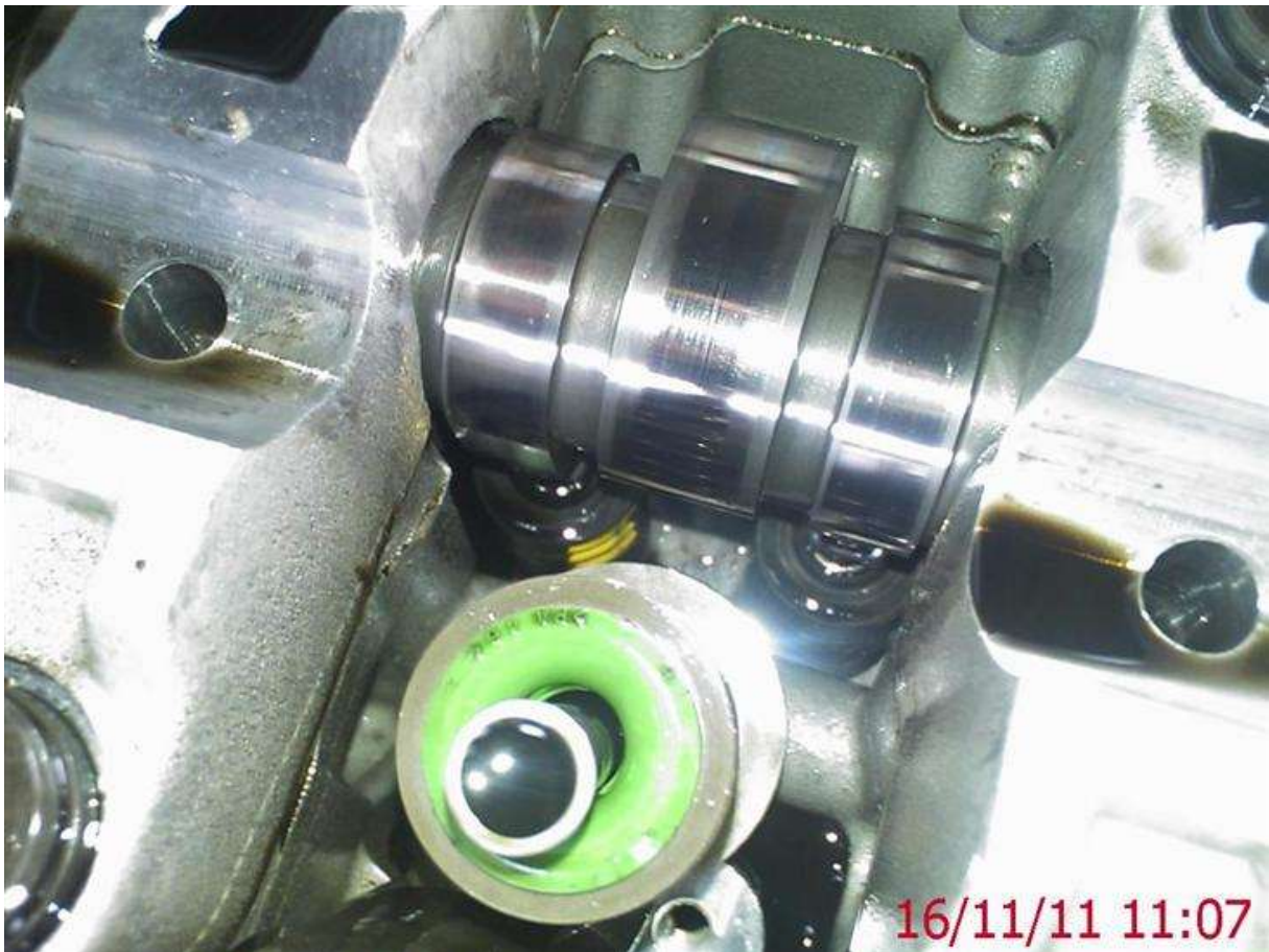
Above you can see the camshaft lobe will "snag" and stop the injector coming out, so remove the camshaft locking pin and rotate the engine until the camshaft lobe is clear from the injector.....
