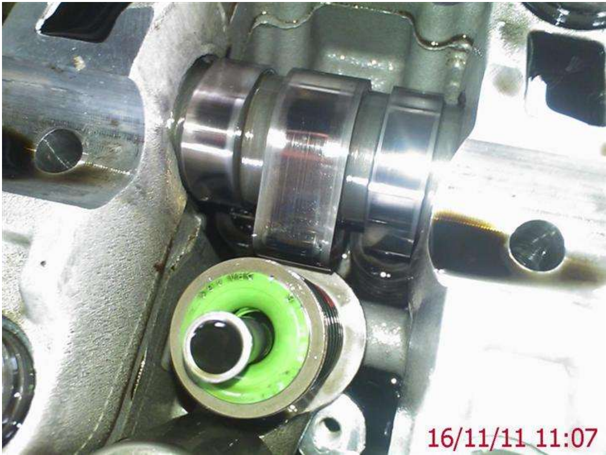
Above you can see the camshaft lobe will "snag" and stop the injector coming out, so remove the camshaft locking pin and rotate the engine until the camshaft lobe is clear from the injector.....
