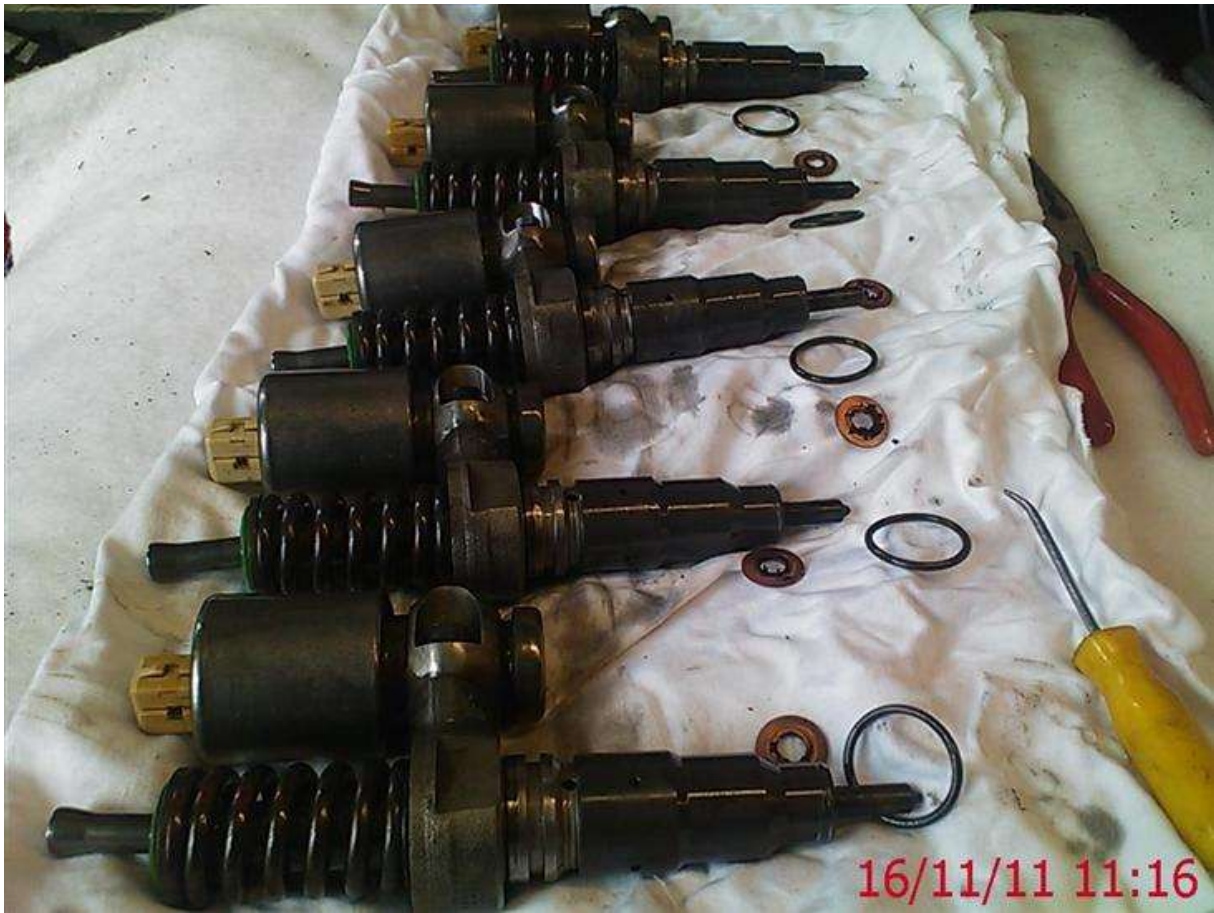
All the "o" rings and copper washers removed, so we have finally got to the bit we want to replace.....
