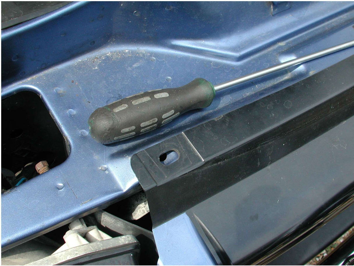
Now remove the self tapping screws from the top lug on both front indicator lamps (circled)
