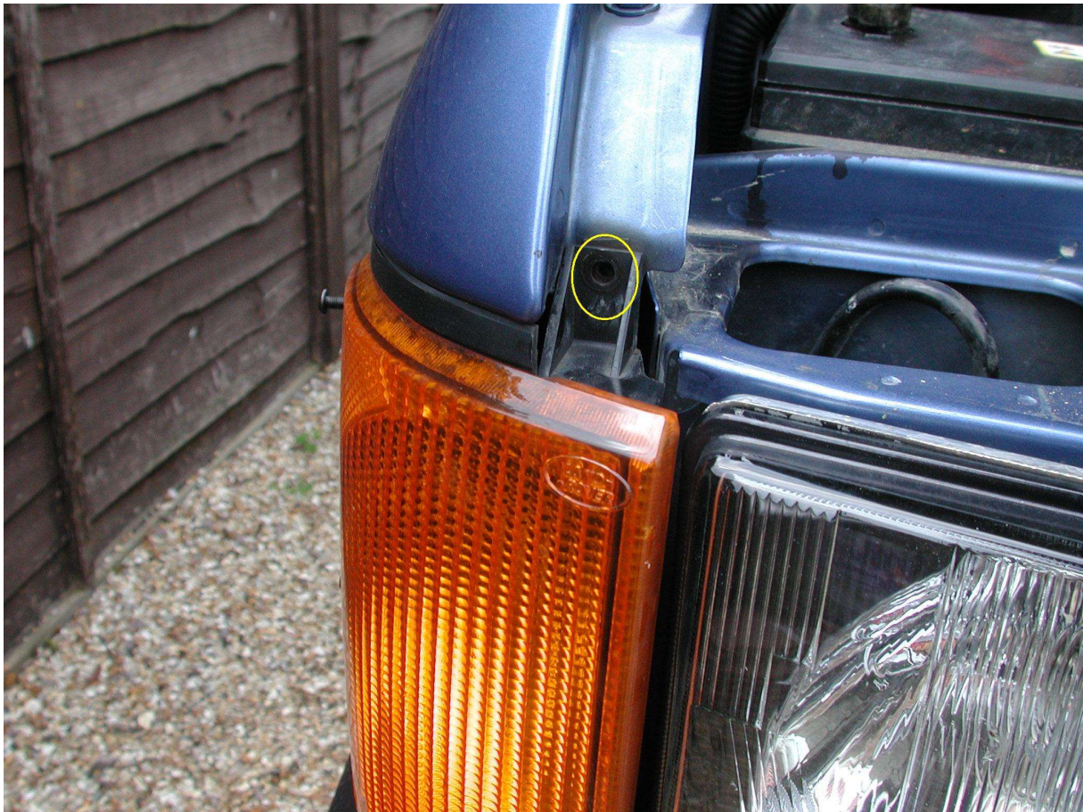
Now remove the self tapping screws from the top lug on both front indicator lamps (circled)
