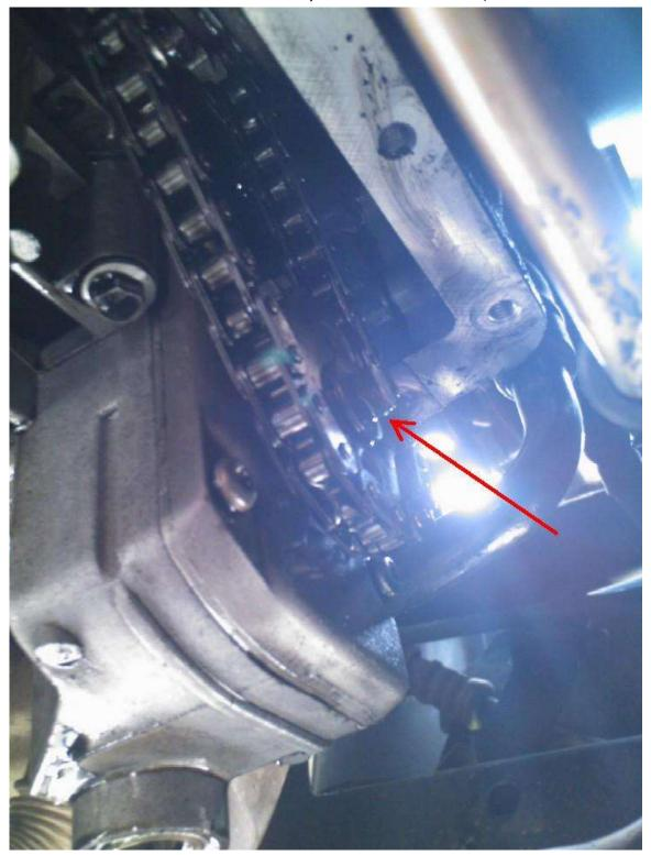
The Pump bolt was superseded by a new part that has thread lock already on it, so its just a case of carefully removing the bolt and installing the new one. Keep hold of the sprocket to make sure it stays in position when you take the bolt out.
