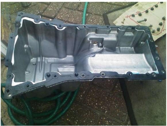
The gasket has molded "dowels" on it to make sure it locates correctly both on the sump and on the bottom of the cylinder block. The gasket is installed DRY.
