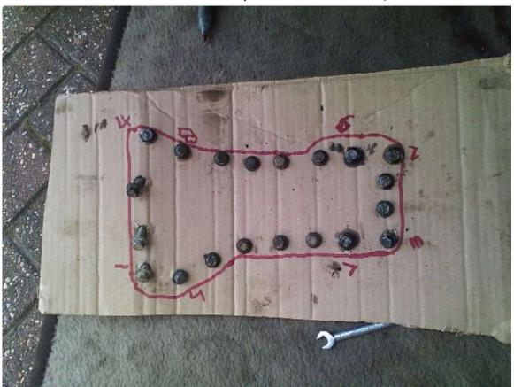
When it comes to the last bolt, remember the sump is cast aluminum so avoid dropping it at all costs, also remember either the 2 bolts or nuts holding the rotor filter drain tube, remove them and manouver the sump down and out to the rear of the car.
