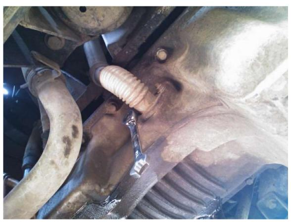
"if" you have nuts, then remove them completely as the pipe will stay sat on the studs and "help" support the sump when you remove it. "If" you have bolts, then it may be a good idea to leave them in just 2 or 3 threads so you can easily remove them by hand when the sump is ready to come off, but they will help support it whilst temporarily left in.
