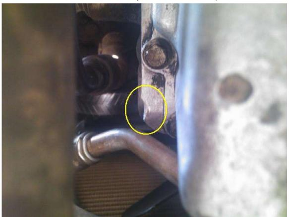
The Pipe is now currently tie-wrapped securely out the way of the sump, once I get a replacement pipe, I will make a bracket and fit a "p" clip to hold it and stop it ever happening again. After writing this article, I did a little research and this is a VERY common issue, although its generally found once it has actually holed the pipe.
