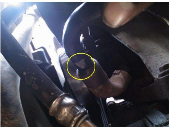
This pipe is a solid metal and rubber pipe. The damage here is at least 50% through the thickness of the metal part of the pipe. Now that have found it and moved it away it would most likely be ok, but I will replace this at the earliest opportunity. Land Rover in their wisdom fitted a pathetic piece of foam to stop this pipe chaffing, but as you can see it didn't really work. A simple bracket and "P" clip would have been the correct way to do it.
