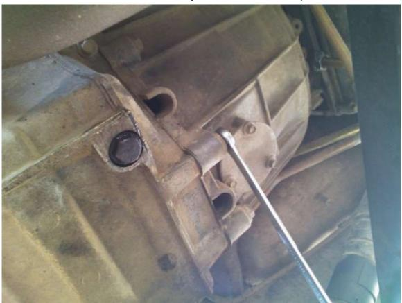
3 can be seen in this picture, the one you cannot see is directly on the opposite side. All 4 of these bolts are the same length / type, but it is good practice to note which one went where for re-assembly later on.
