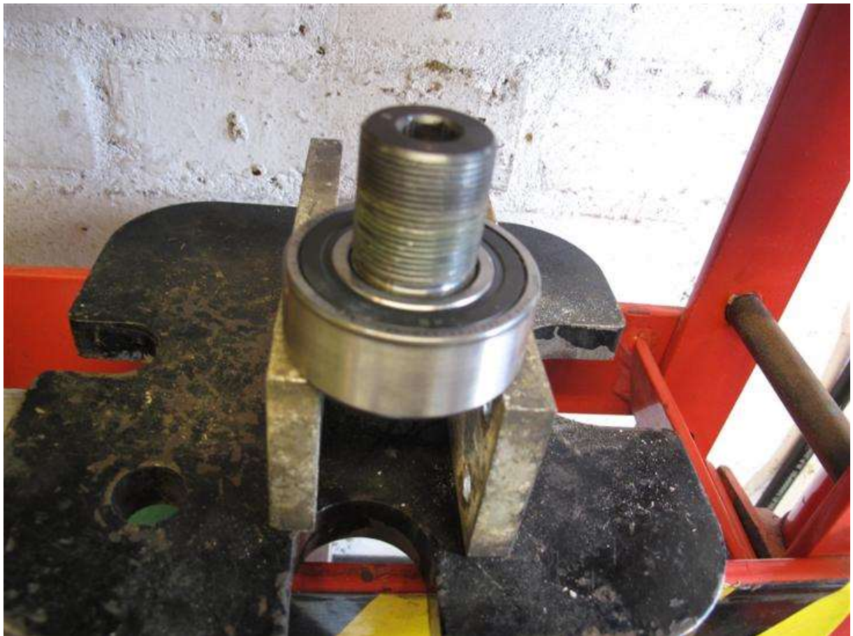
New bearing fitted to the shaft below.... it simply goes all the way in till the shoulder of the shaft is against the bearing...
