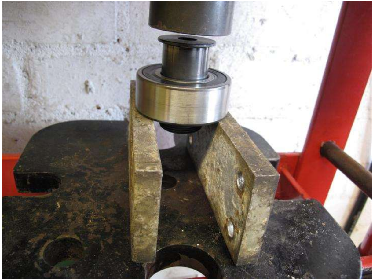
New bearing fitted to the shaft below.... it simply goes all the way in till the shoulder of the shaft is against the bearing...
