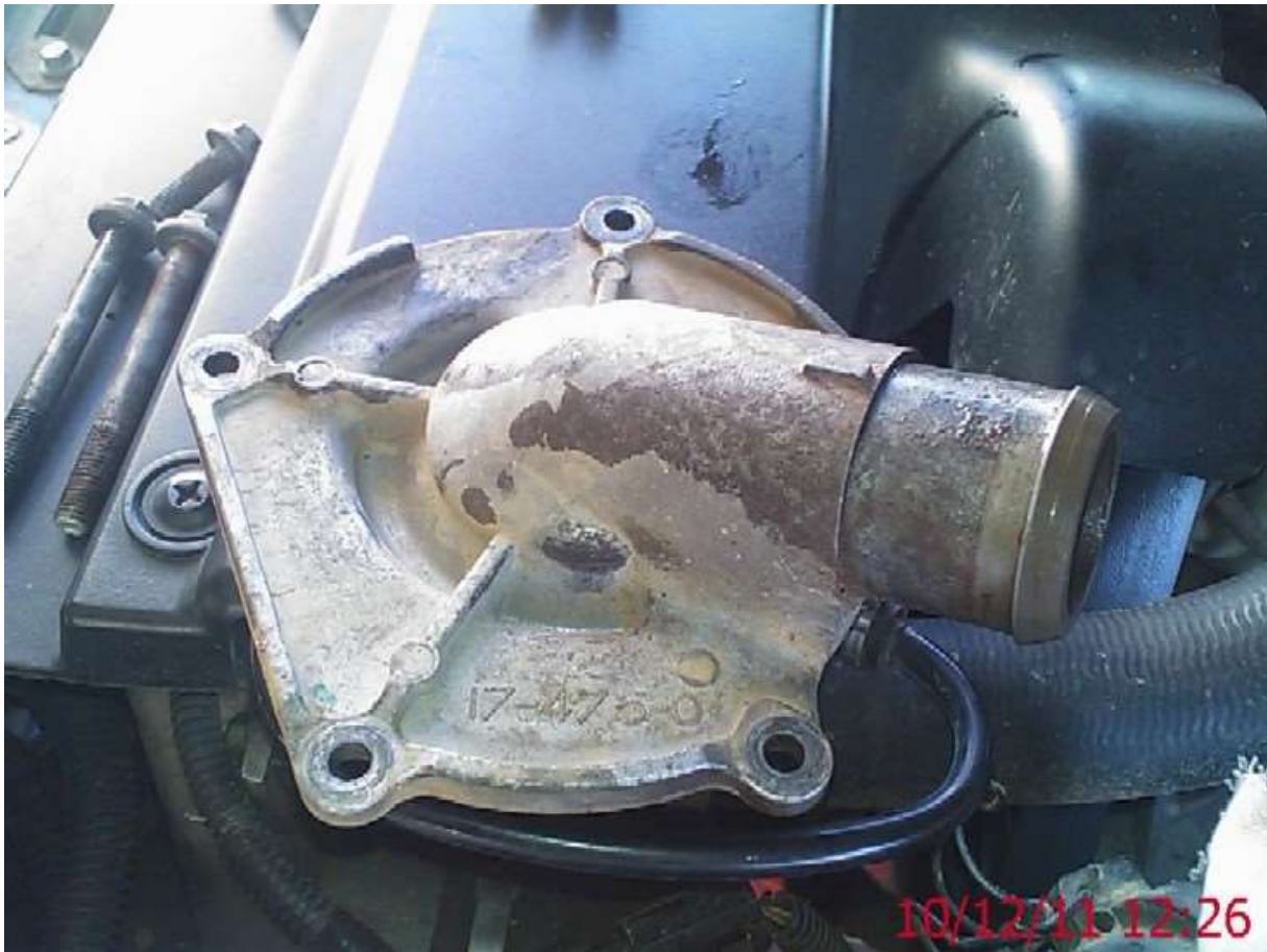
This reveals the water pump.
