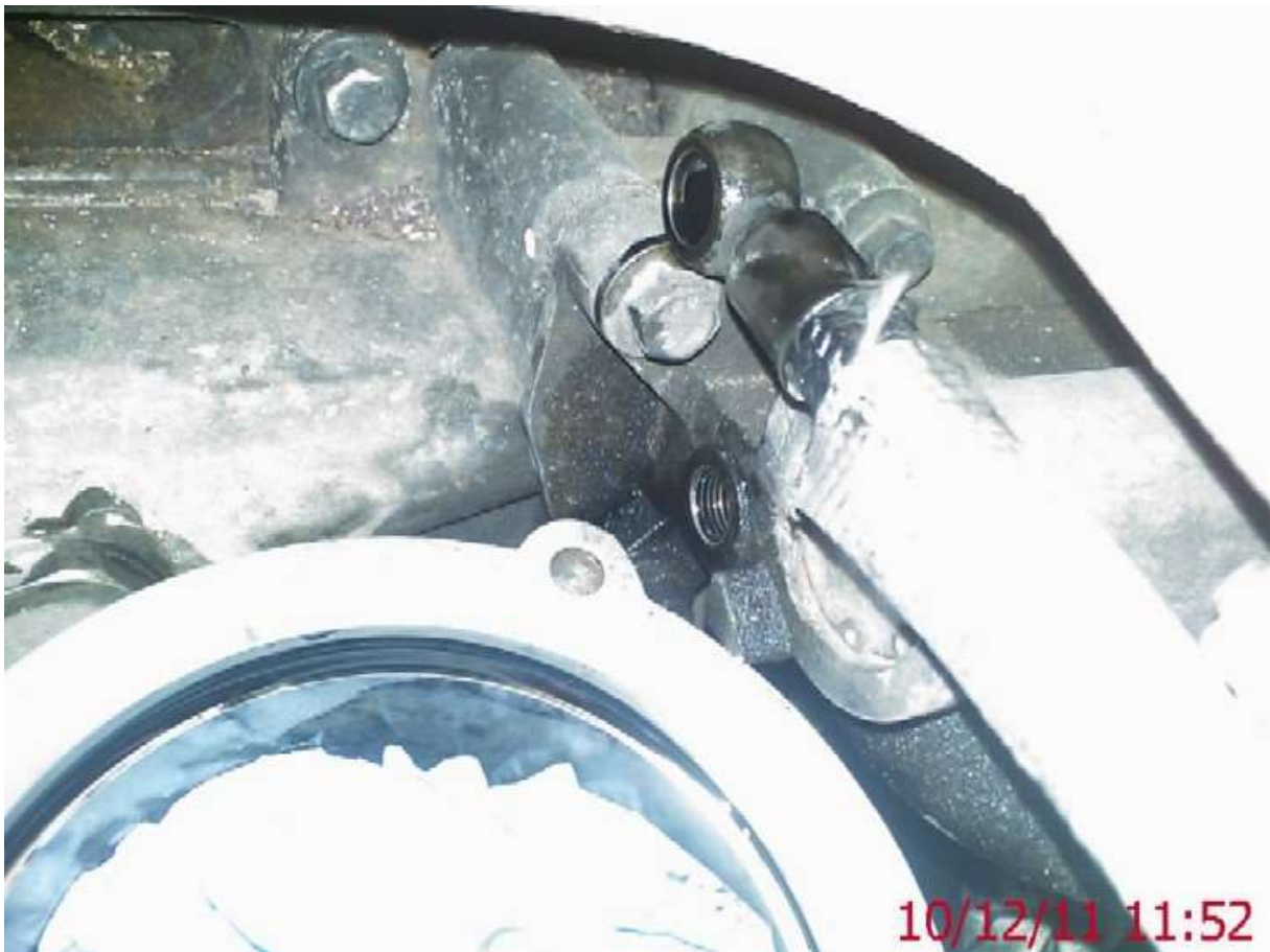
Turbo oil feed hose banjo removed (above), one washer stuck under the head still and the other from the housing side.. Once removed, then flex the hose up and clear of the rotor housing..
