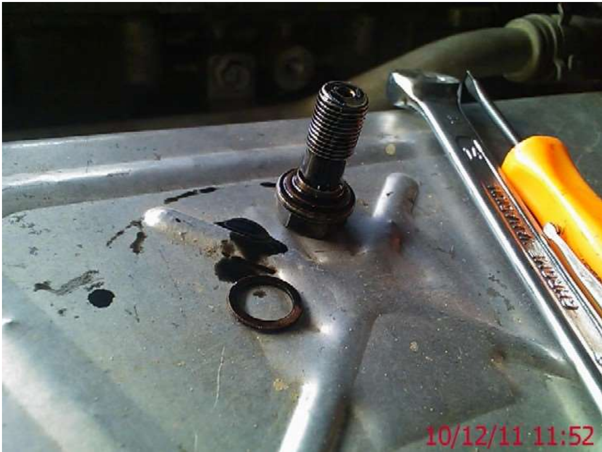
Turbo oil feed hose banjo removed (above), one washer stuck under the head still and the other from the housing side.. Once removed, then flex the hose up and clear of the rotor housing..
