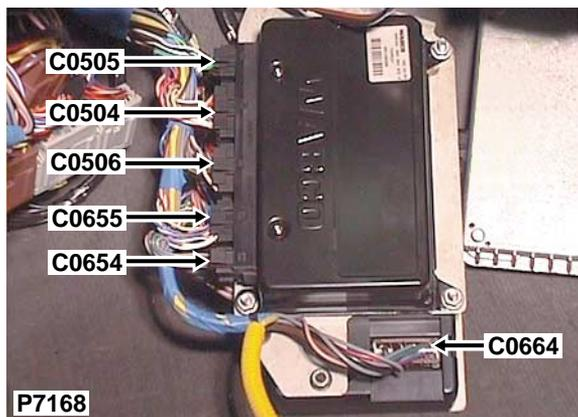
Description: *ECU-Self-levelling/ABS (SLABS)*
