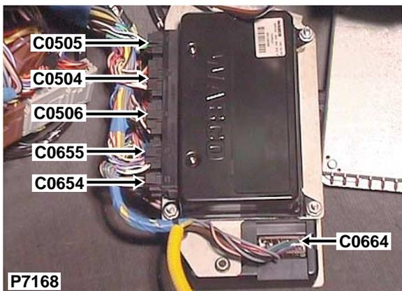
Description: *ECU-Self-levelling/ABS (SLABS)*
