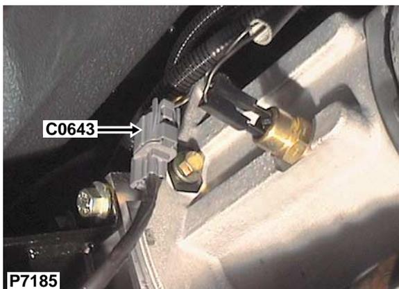
Description: *Sensor-Heated oxygen (HO2S)-Rear-LH*
